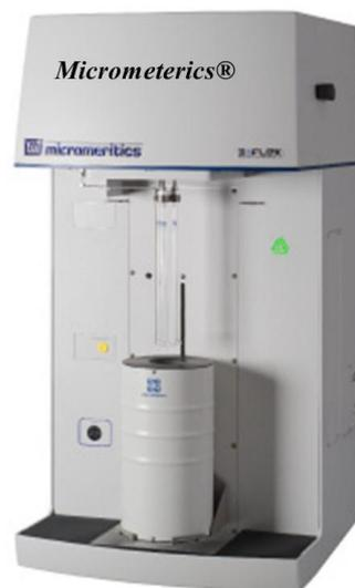
Figure 141 : Appareil de physisorption Micromeritics, Norcross, GA, USA.
