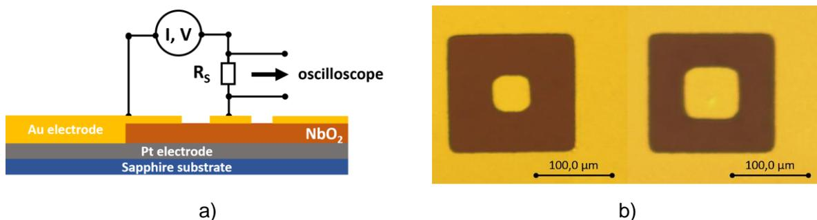
Figure 93. Schematic of the metal-insulator-metal vertical NbO<sub>2</sub> device and the associated electrical setup for MIT activation and b) top view of an MIM device with upper electrodes of 50 μm (left) and 70 μm (right) lateral size.
