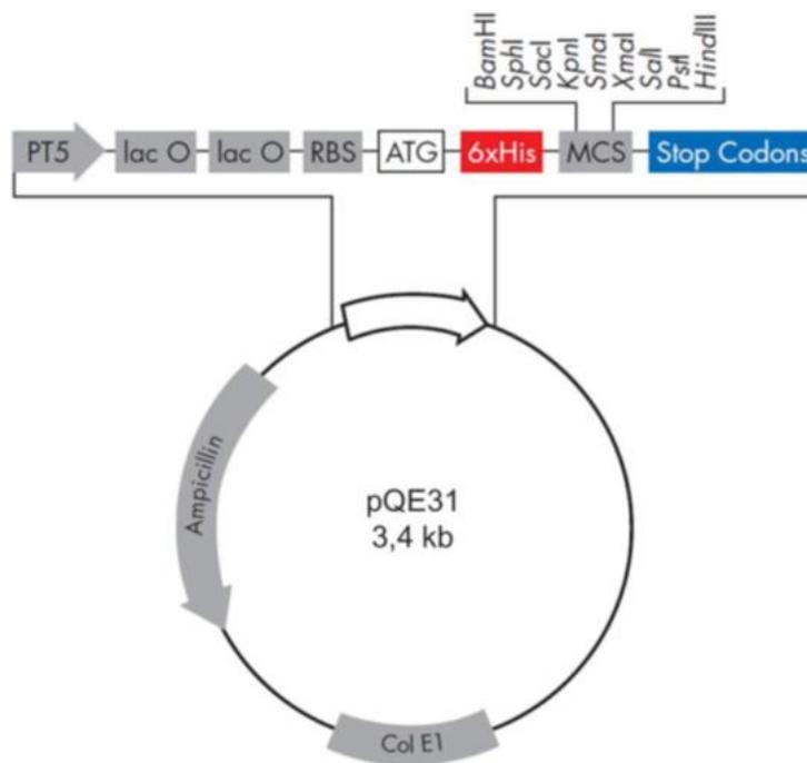
**Figure M-4. The map of pQE-31 vector used for the insertion of OBP56d or OBP56g coding region.**
