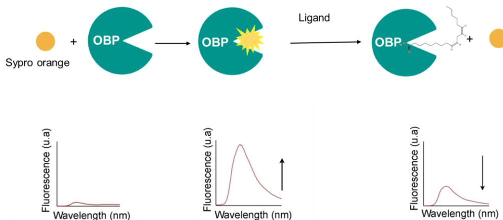
**Figure M-8. Principle of the fluorescent binding assay**
