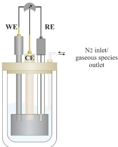
Figure 3.5. Schematic representation of the electrochemical setup utilized for AWE application essays.
