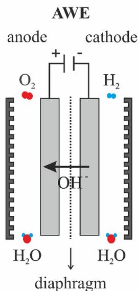
Figure 2.5. Schematic illustration of Alkaline Water Electrolysis setup.
