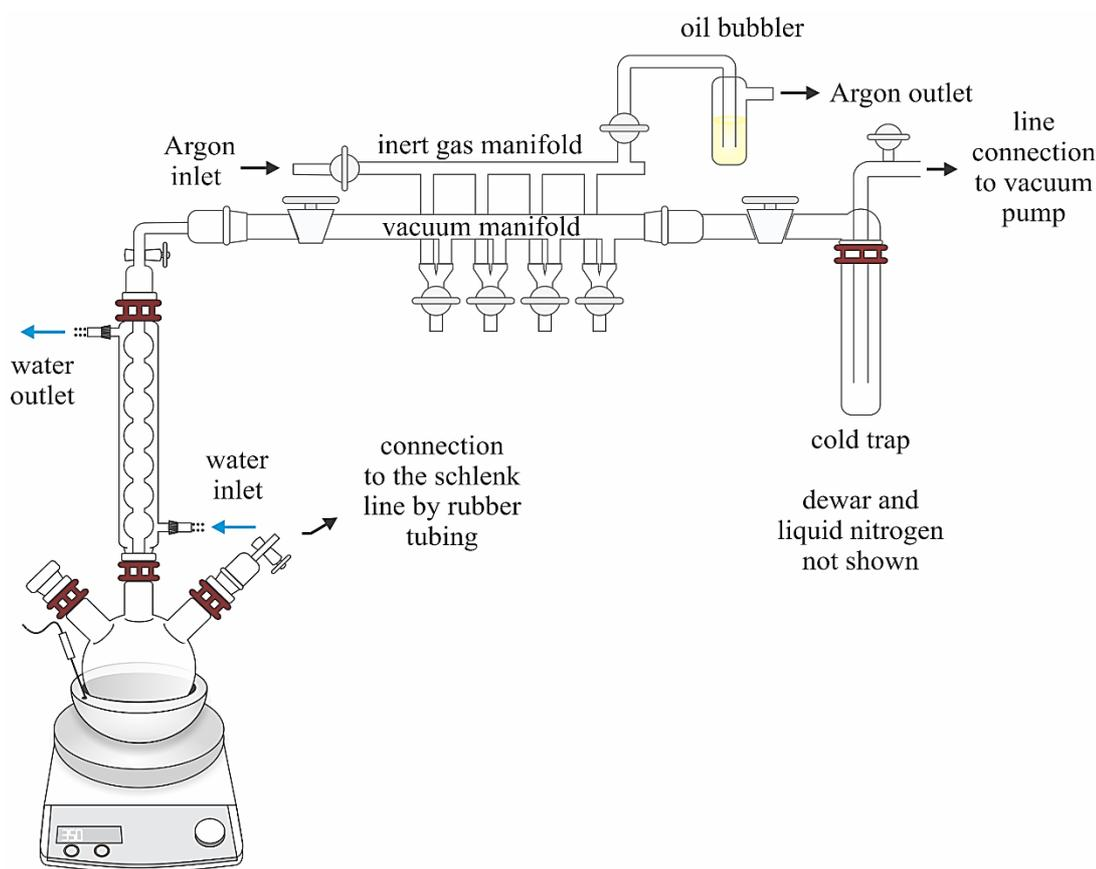
Figure 3.3. Schematic representation of a Schlenk line.
