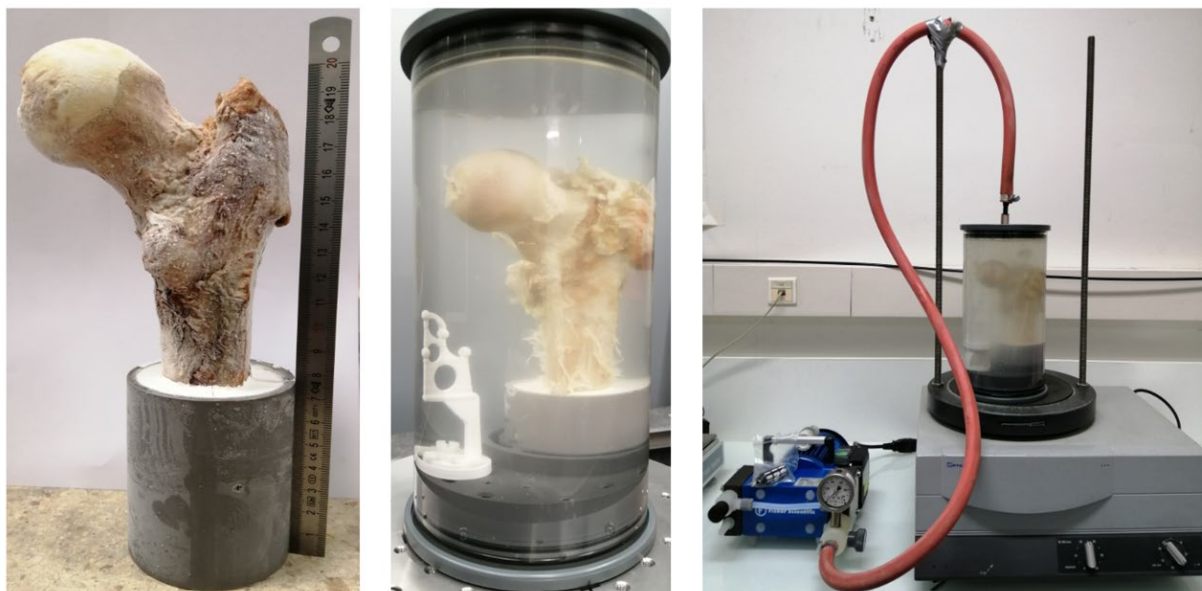
Figure 4. 2: Sample preparation setup. First Fresh sample (S05) preparation. a.(left) unfrozen femur head. b.(middle) cylindric plastic jar filled by 1mM Gd-DTPA saline solution with 3D-printed tool (bottom left) used for 3D volumes registration. c. (Right) vacuum pump and vibrating surfaces.
