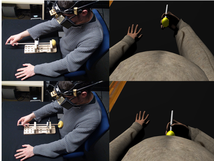
Figure 2.6 – Illustration from the study of Normand et al. [2011]. Whenever participants poke their belly with the rod, the virtual belly is touched at the same time by the virtual rod. It therefore provides synchronous multisensory stimulation towards the larger virtual body.
