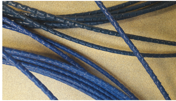
FIGURE 2.46: V9 F ▲ type samples before (bottom) and after (top) exposure to the temperature cycle. The temperature impact reveals that the absorbed radiation darkened the cable.
