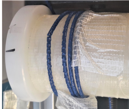
FIGURE 2.22: Impact of the radiation on the V9 type cable: radiation reduces the ductility of the plastic, causing cracks when curved.
