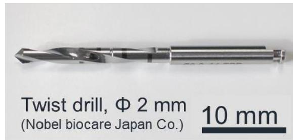
Fig. 2-6 Twist drill bit used for a series of drill tests
