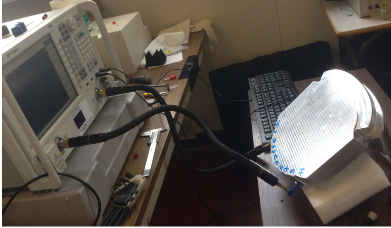
Figure 4.21: Setup for the measurements of the S-parameters
