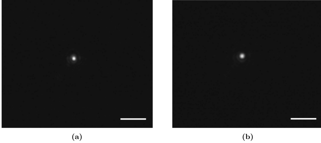
Figure 5.7 Focal spot after the complete integration. Focal spot created by the integrated probe at 800 nm (a) and 1040 nm (b) of the laser beam propagated through the probe's NCF. Scale bar: 10 \mu\text{m} .
