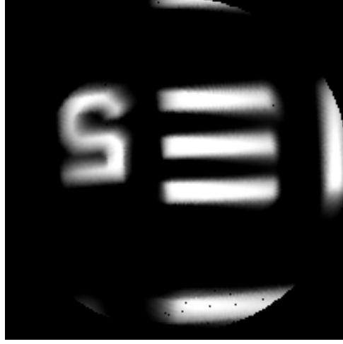
Figure 5.8 USAF-1951 negative transmission chart imaging (group 5, element 5).
