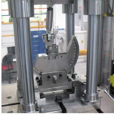
(a) Peeling load at an angle of 0^\circ/0^\circ .
