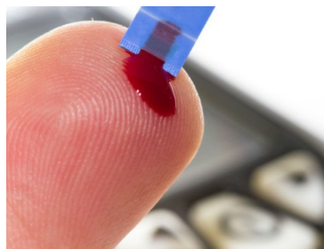
Figure 11: Picture of the blood from the fingertip conducted a glucometer. The glucometer device is a qualified as a microfluidic device: Blood is transported to the device by capillarity through a plastic test strip. The glucose concentration in the blood is indicated on the device screen.
