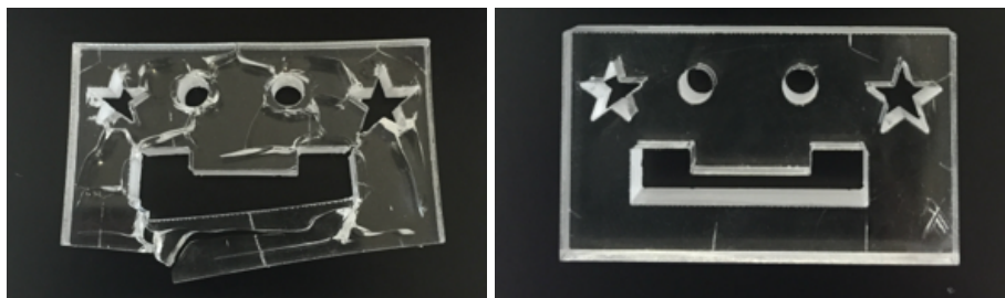
Figure 18: Pictures of PMMA blocks cut using a CO 2 laser-cutter (Speedy 100, Trotec, Austria). The PMMA on the left side was untreated and the PMMA on the right side was heated at 90°C for two hours after being cut. Both PMMA blocks were placed in acetone for two hours. The pre-heated PMMA block showed improved chemical resistance. The few visible marks on the pre-heated PMMA are due to the honeycomb of the laser-cutting machine.
