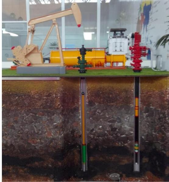
*Figure 5. Reservoir, production tubing and surface facilities in a crude oil production site. Two wells are represented one with mechanical pump recovery and the other producing by natural reservoir pressure reduction. X-tree, three phase separator and stocking units are also shown. (Photo taken at the stand of the China Petroleum Technology Development Corporation, CPTDC at Rio Oil and Gas 2014).*
