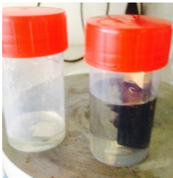
Figure 2.17: Platinum (left) and gold (right) during test with DMF
