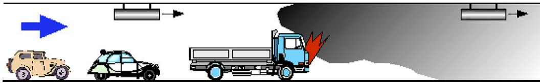
Fig. 1.1 Fire-induced smoke longitudinal control (Vauquelin, 2008).
