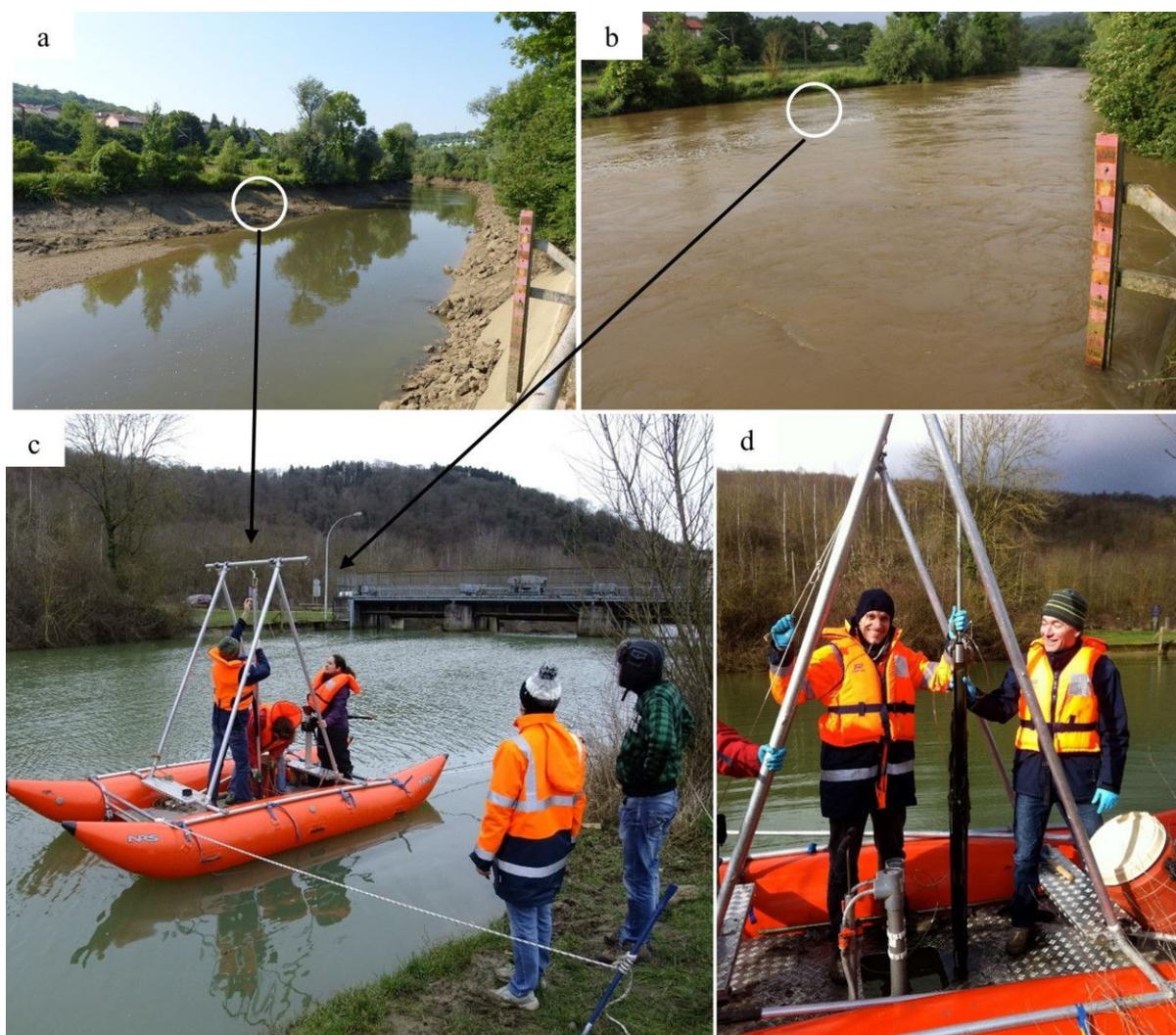
Figure II-19: The area upstream the Beth dam, Moyeuve-Grande, and collection of a sediment core using a floating platform (quadri-raft).
