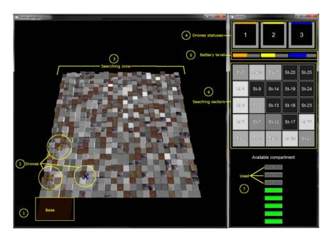
Figure 6.1: Operator's graphical interface.
