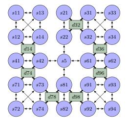
Figure 5.1: Topological model with the points of interest and all possible transitions. Figure 5.2 shows a moment during the mission with three drones. In this simulation, the
