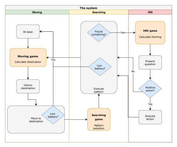
Figure 8.1: Flowchart of a typical mission.
