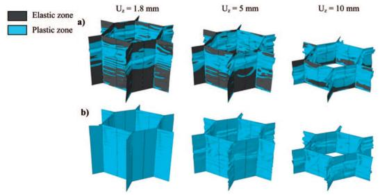
Figure I-18: Écrasement d'un nida aluminium (a) 12 m/s and (b) 120 m/s [Kolo13]
