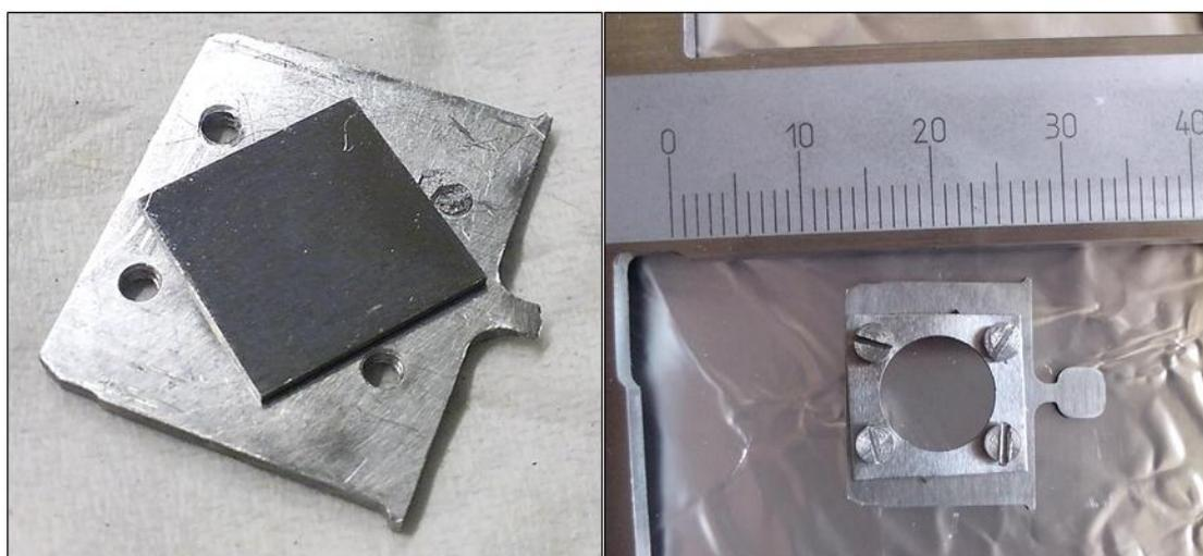
*Figure 13 – A PW sample with a broken grabbing key (left); A PW sample mounted on the transfer platen (right)*
