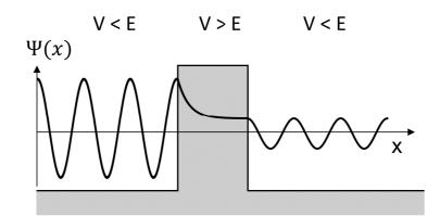
Figure 1.3: **Tunneling effect:** Simple case of a free electron encountering a rectangular potential.
