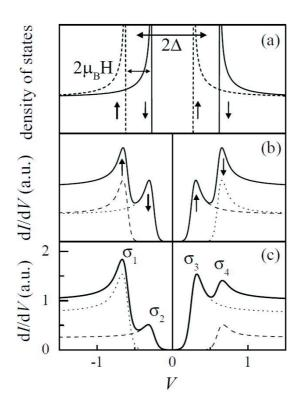
Figure 1.5: **Spin-dependent tunneling:** Panel (a) represents the Zeeman-split density of states of a superconducting layer. Panel (b) depicts the expected conductance spectra of unpolarized electrons from a metal to a superconducting layer. Panel (c) shows the conductance from a ferromagnet to a superconducting layer. See text for more details. Figure adapted from LeClair<sup>35</sup>.
