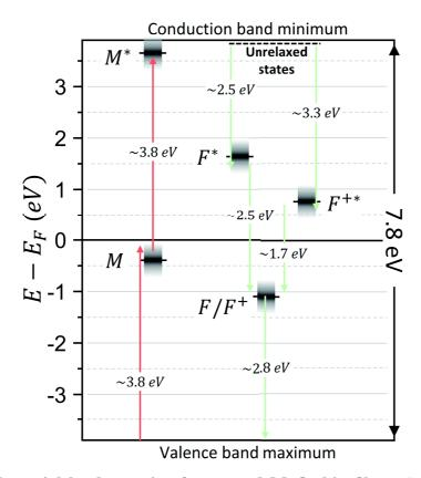
Figure 4.3: **Potential landscape in rf-sputtered MgO thin films:** Potential landscape in rf-sputtered MgO proposed by Schleicher *et al.*<sup>190</sup>. Differences between this diagram and the potential landscape proposed in this thesis (see Figure 4.1) are detailed in the text.
