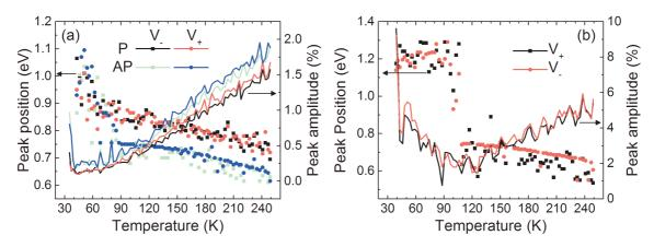
Figure 4.10: **Peak positions and amplitude:** Peak position and amplitude extracted from (a) P and AP  $\hat{I}_{rel}$  datasets and (b) the TMR relative thermal drop. Data for both positive and negative bias voltage are shown. We remind that the position of  $\hat{I}_{rel}$  peaks corresponds to the energy position of a thermally activated process.
