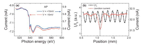
Figure 6.4: Synchronized measurements: (a) Raw data of current flowing through the MTJ while sweeping the energy of photons with linear vertical polarization across the O K edge for (left) negative bias voltage -10 mV, and (right) positive bias voltage 10 mV. Note a strong variation beginning at ~ *S1535eV* due to the generated photocurrent, which is of negative sign in both cases. (b) The motors' position and the resistance can also be synchronized and used to align the sample with precision.
