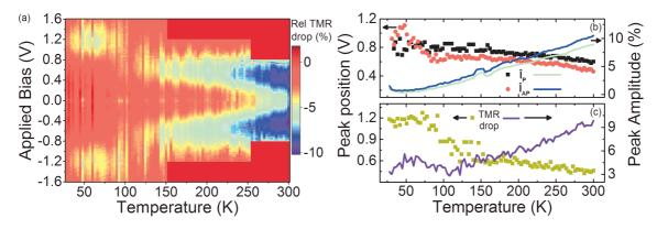
Figure 4.11: Extended dataset of the magnetoresistive properties in the (V,T) parameter space: (a) 2D color map of the TMR relative thermal drop in the (V,T) parameter space, (b) peak maximum position and amplitude extracted from  $\hat{I}_{rel}$  for both magnetic states and (c) peak maximum position and amplitude of TMR relative thermal drop. Extended dataset measured between 16 K and 300 K.
