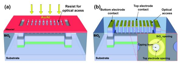
Figure 3.4: **Step IV, Metalization:** Schematic view of (a) sample with resist defining top electrode openings on pillars for optical access and (b) sample after metal deposition and lift-off. The inset of panel (b) represents a top view of the optical access on the pillar.
