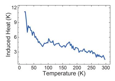
Figure 5.8: **Heat induced by 3.05 eV photons excitation:** Heat induced by laser excitation as a function of the sample's temperature. See text for more details.
