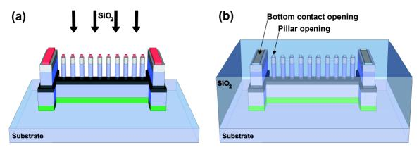
Figure 3.3: Step III, Passivation layer deposition: Schematic view of (a) sample with resist defining  $SiO_2$  openings on pads and pillars for electrical contact and (b) sample after  $SiO_2$  deposition and lift-off.
