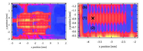
Figure 6.2: **MTJ alignment with the x-ray beam:** Example of mapping a sample containing MTJs using x-ray absorption at 788 eV (Co  $L_3$  edge). (a) Large-scale map of the sample on the chip with the region of interest (containing 20 MTJs) within a yellow rectangle. (b) Fine alignment of the junction with (1) bottom electrode pad, (2) top contact and (black "x") the exact position of the MTJ of interest. Dark areas represent the regions covered by metal thus with attenuated x-ray absorption.
