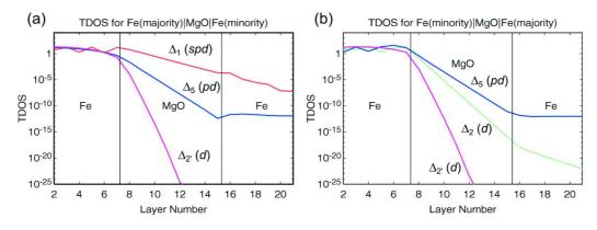
Figure 1.13: Fe/MgO/Fe tunneling DOS in the antiparallel magnetic state: Panels (a) and (b) represent the tunneling DOS in the antiparallel magnetic configuration for  $G^{\uparrow\downarrow}$  and  $G^{\downarrow\uparrow}$  respectively. See text for more details. Figure adapted from Zhang and Butler<sup>49</sup>.
