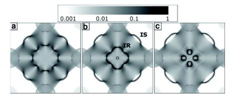
Figure 2.2: Fe (001)  $k_{\parallel}$ -resolved minority DOS: Minority DOS of the topmost Fe layer in a Fe/MgO/Fe (001) trilayer for three energies: (a) 0.02eV below  $E_F$  (b) at  $E_F$  and (c) 0.02eV above  $E_F$ . Regular surface states and resonance states are maked IS and IR respectively. Figure reproduced from Belashchenko *et al.*<sup>72</sup>.
