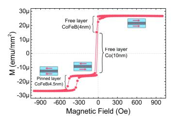
Figure 4.4: **Magnetic properties of samples before optical lithography:** All magnetic layers in our samples have in plane magnetization with the same easy axis direction. We can see that the Co(10 nm) and CoFeB(4 nm) free layers are reversed at small negative applied magnetic fields. The CoFeB(4.5 nm) electrode on top of the IrMn(7.5 nm) antiferromagnetic layer is exchange biased and switches at larger applied magnetic fields.
