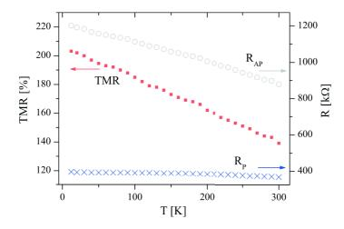
Figure 2.19: **Temperature dependence of electrical transport in MgO based MTJs:** The resistance of both P and AP magnetic state as well as TMR as a function of temperature in exchange biased CoFeB/MgO/CoFeB MTJs. The TMR decrease is principally due to the strong decrease of  $R_{AP}$ . In comparison  $R_P$  is almost temperature independent. Reproduced from Drewello *et al.*<sup>113</sup>.
