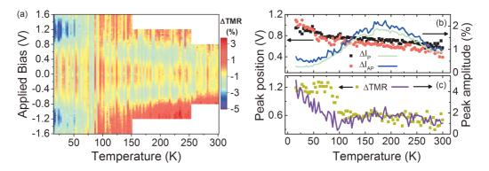
Figure 5.4: Impact of 3.05 eV linearly polarized light on bias- and temperaturedependent transport properties: (a) 2D color map of the TMR drop induced by 3.05 eV photons excitation in the (V,T) parameter space, (b) peaks position and amplitude extracted from  $\Delta I_{\sigma}(V,T)$  for both P and AP device magnetic state and (c) peak position and amplitude of TMR drop extracted from panel (a).
