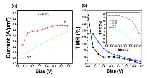
Figure 2.8: **Impact of interface disorder in the non-equilibrium regime:** Conductance (a) and TMR (b) as a function of bias voltage for various x, the proportion of atoms moved from the right electrode interface to the left electrode interface. See text for more details. Figure reproduced from Ke *et al.* <sup>93</sup>.
