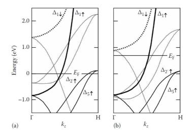
Figure 1.15: **Spin- and symmetry-resolved band structure of bcc Fe and Co:**  $\Delta_5$  and  $\Delta_{2'}$  are present in both majority and minority spin population of bcc Fe electrodes while they are totally spin polarized in bcc Co. This is expected to further reduces  $G_{AP}$  increasing the conductance asymetry between P and AP and the resulting TMR. Figure taken from Tsymbal and Zutic<sup>41</sup>.
