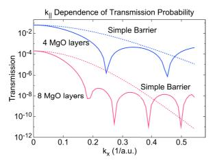
Figure 1.14: **Interference of tunneling states:** Tunneling DOS as a function of  $k_x$  for  $k_y = 0$ . The LKKR decay rate (solid lines) is compared to the simple barrier model (dashed lines) for 4 and 8 MgO monolayers (blue and red respectively). The oscillatory dependence of the TDOS can't be explaind by simple models. Figure adapted from Zhang and Butler<sup>49</sup>.
