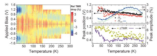
Figure 5.9: Impact of 0.8 eV linearly polarized light on bias- and temperaturedependent transport properties: (a) 2D color map of the TMR drop induced by 0.8 eV photons excitation in the (V,T) parameter space, (b) peaks position and amplitude extracted from  $\Delta I_{\sigma}(V,T)$  for both P and AP device magnetic state and (c) peak position and amplitude of TMR drop extracted from panel (a).
