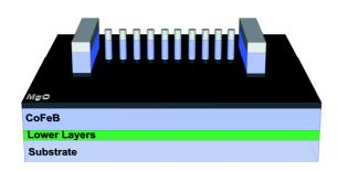
Figure 3.1: **Step I, Pillar definition:** Schematic view of (a) lithographic mask with desired pattern in contact with resist previously deposited on top of the sample and UV insulation step (b) sample etching after resist development and (c) sample after lift-off and cleaning in ultrasonic bath. Note that not all layers are shown and that picture is not to actual scale.
