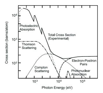
Figure 3.10: **Cross sections of light-matter interactions:** Cross section of the photoelectric absorption, Thomson and Compton scattering, electron-positron pairs creation and photomolecular absorption as a function of photon energy. Within the soft X-ray range, the photoelectric absorption is order of magnitude higher than other processes. Figure taken from C. Felix's thesis<sup>204</sup>.
