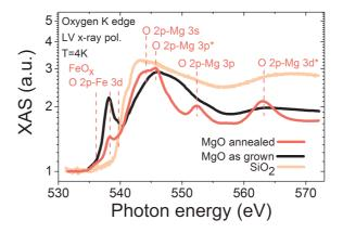
Figure 6.3: **Reference XAS spectra:** XAS O K edge reference spectra of as-grown and annealed MgO, and SiO<sub>2</sub>. The peak identification is based on the literature and reflects the allowed transitions from oxygen 1s core to final states assigned in  $red^{219,220}$ .
