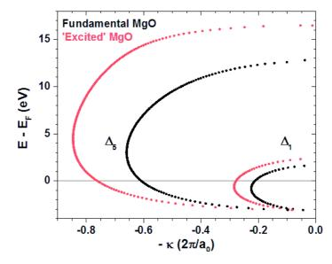
Figure 6.7: **Complex band structure of MgO under x-ray excitation:** Complex band structure of MgO in its fundamental (black) and excited (red) states. Excited MgO is modeled by replacing all the O atoms by F atoms. This could artificially increase the band gap and the complex loop amplitudes, we nevertheless observe an increase in  $\kappa_5$  that is much larger than for  $\kappa_1$ .
