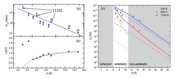
Figure 2.32: **Tunneling between oxygen vacancies in MgO:** (a) Electronic coupling matrix elements and (b) reconfiguration energy as a function of the distance d between F centers along various crystal directions. (c) Electron transfer rate betwenn oxygen vacancies as a function of d in MgO plotted for three temperatures. Dashed lines are calculated assuming nonadiabatic electron transfer and constant activation energy. Reproduced from McKenna and Blumberger<sup>185</sup>.
