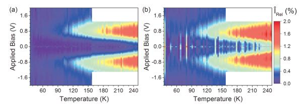
Figure 4.8: Bias and temperature dependence of the tunnel current in the parallel and antiparallel magnetic configurations: Following Rottlander's technique and using Equation (4.1),  $\hat{I}_{rel}$  is computed for both P and AP magnetic states and plotted in panels (a) and (b) respectively. We can see that a dominant peak impacts both P and AP conductance at 0.8 eV. Both the bias position and amplitude of the peak are extracted from these datasets and plotted in Figure 4.10(a).
