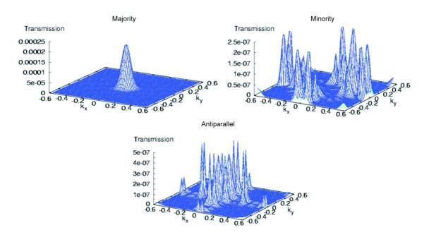
Figure 1.9: Distribution of conductance as a function of  $k_{\parallel}$ :  $k_{\parallel}$ -resolved conductance for eight monolayers of MgO. Conductance in the parallel magnetic configuration for majority and minority spin channels are represented in top right and top left panels respectively. Conductance in the antiparallel configuration is shown in the bottom panel. See text for more details. Figure adapted from Butler *et al.*<sup>44</sup>.
