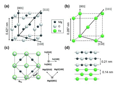
Figure 1.7: **Structure of the Fe/MgO (001) interface** The Rock-salt and the bcc crystal structure of MgO and iron are shown in panel (a) and (b) respectively. Top view and cross section of the Fe/MgO(001) interface are schematized in panel (c) and (d). We can see that MgO[100] is parallel to Fe[110]. Figure adapted from Yuasa and Djayaprawira<sup>45</sup>.
