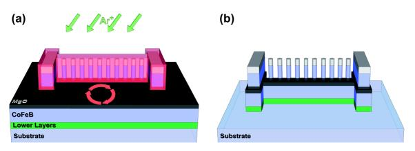
Figure 3.2: **Step II, Bottom electrode definition:** Schematic view of (a) sample with resist defining the bottom electrode (UV insulation step not shown) as introduced in the etching chamber and (b) sample after etching, lift-off and cleaning in ultrasonic bath.
