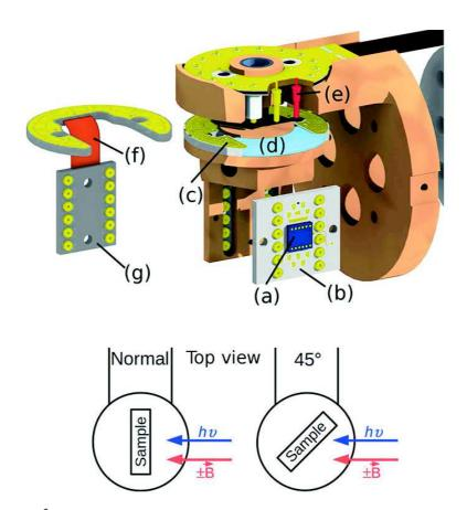
Figure 3.12: **V<sup>2</sup>TI immediate sample environment:** (a) sample (dark blue), (b) sample PCB chip ready to be plugged in (g), (c) 12 electrical contacts, (d) teflon part, (e) spring dot, (f) kapton flex, (g) sample holder PCB. Bottom: top view sketch showing direction of photon and direction of magnetic field for both 0 ° and 45 °working positions. Figure taken from Joly *et al.* <sup>206</sup>.
