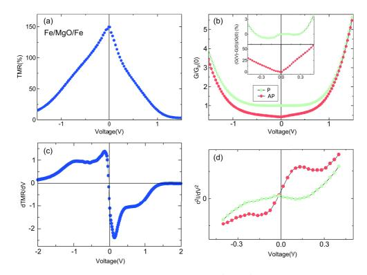
Figure 2.4: **Magnetotransport properties of Fe/MgO/Fe with clean interfaces:** TMR and its derivative are plotted in panels (a) and (c). The normalized conductance and current second derivative are plotted in panels (b) and (d) respectively. See text for more details. Figure taken from Tiusan *et al.*<sup>82</sup>.
