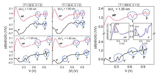
Figure 2.18: **Impact of trap states on IETS in CoFeB/MgO based MTJs:** (a) and (b) plot IETS spectra measured at low temperature for positive and negative bias voltage for  $t_{MgO} = 1.05$  nm. (c) and (d) plot similar data for  $t_{MgO} = 1.35$  nm for which additional room temperature measurements are presented in panel (e). Clear signature of trap states are emphasized with blue circles. See text for more details. Reproduced from Teixeira *et al.*<sup>138</sup>.
