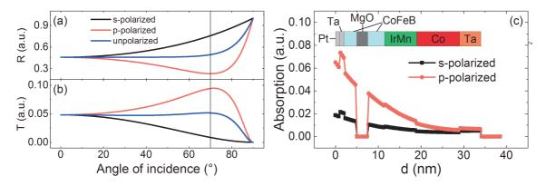
Figure 5.7: **Reflection, transmission and local absorption of 3.05 eV p- and spolarized light:** The proportion of reflected and transmitted light for both polarization are plotted in panels (a) and (b), respectively. The local absorption as a function of the depth in the multilayer stack is ploted in panel (c). These quantities are computed as unitless fraction of the total incoming power.
