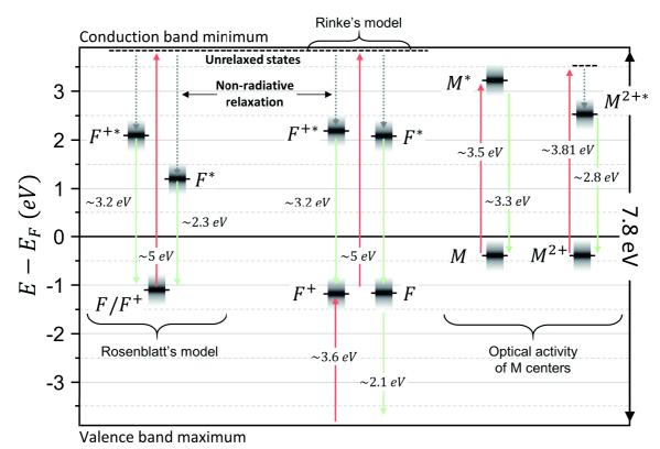
Figure 4.1: **Optical activity of MgO:** This figure summarizes absorption and emission peaks induced by F and M center in MgO. Two models for the emission of F centers, discussed in Section 2.4.3, are represented. Additionally, the photoluminescence of M and  $M^{2+}$  is also represented. Table 4.1 summarizes the absorption
