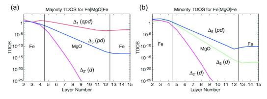
Figure 1.12: **Fe/MgO/Fe tunneling DOS in the parallel magnetic state:** Panels (a) and (b) plot the tunneling DOS as a function of the position in the Fe/MgO/Fe trilayer in the parallel magnetic state, for majority  $(G^{\uparrow\uparrow})$  and minority  $(G^{\downarrow\downarrow})$  channels respectively. There is no  $\Delta_1$  channel in the minority channel. See text for more details. Figure adapted from Zhang and Butler<sup>49</sup>.
