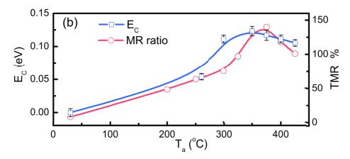
Figure 2.17: Magnon activation energy and TMR as a function of annealing temperature in CoFeB/MgO based MTJs: An apparent correlation is visible between magnon activation energy  $E_c$  and TMR. TMR increases with magnon activation energy, suggesting that magnon have a strong impact on magnetotransport properties. Reproduced from Ma *et al.*<sup>122</sup>.
