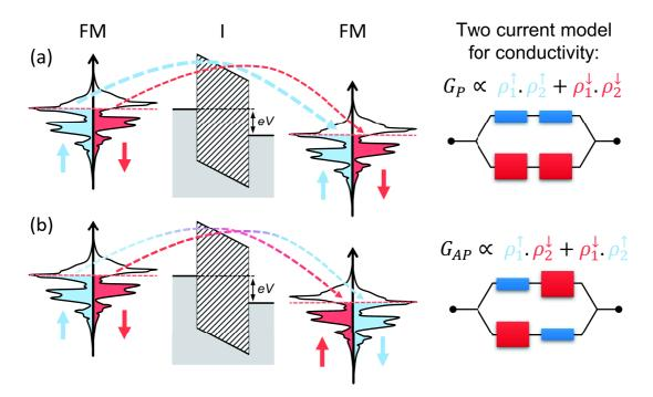
Figure 1.6: **The Jullière model for TMR:** The figure represents electrons tunneling between ferromagnetic (FM) electrodes through an insulating layer represented by a potential step (striped area) when a bias V is applied to the magnetic tunnel junction. Both parallel and antiparallel magnetic states are represented in (a) and (b) respectively. The model is based on two hypothesis that allow to apply the two current model (represented on the right hand side). See text for more details.
