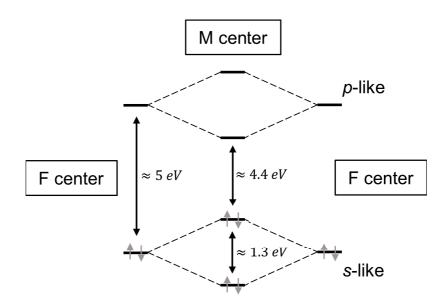
Figure 2.31: **Optical activity of double oxygen vacancies:** Simple representation of the energy levels involved in the electronic excitation of M centers (double oxygen vacancies). Adapted from Domínguez-Ariza *et al.*<sup>181</sup>.
