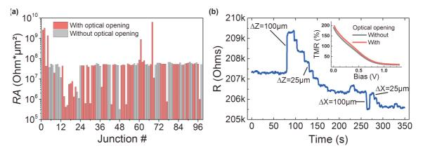
Figure 5.2: Basic magneto-electric properties and alignment procedure: (a) RA product of MTJs with and without optical opening on the same chip. (b) Examples of aligning the 2.6 eV source by following the evolution of resistance for V = 10 mV and T = 33 K during the two-axis displacement sweep. The inset of panel (b) plots the bias dependence of TMR for MTJs with and without optical opening.
