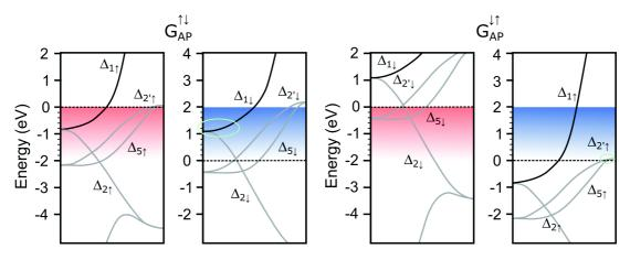
Figure 2.11: Impact of bias voltage related to the band structure of the ferromagnetic leads: Similar drawing as Figure 2.10 for the AP magnetic state. See text for more details.
