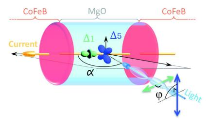
Figure 5.1: Geometry of optical excitation: A current with dominant  $\Delta_1$  or  $\Delta_5$  electronic symmetry tunnels between electrodes (red) across MgO (transparent blue). The photon impinges the device at an angle  $\alpha$  relative to the MTJ normal. The angle between the direction of junction current *I* and the light's electric field is denoted  $\phi$ .
