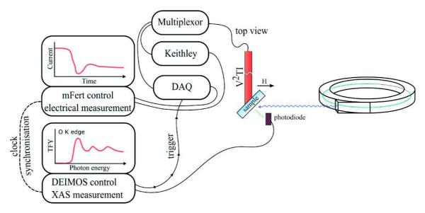
Figure 6.1: **Experimental setup:** X-ray photons interact with an operating device. Simplified schematic of the experimental setup combining the magnetotransport bench and DEIMOS beamline end-station control.
