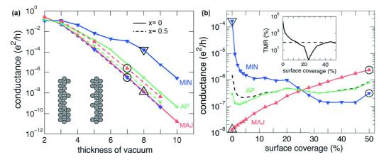
Figure 2.7: Impact of interface disorder in the equilibrium regime: Conductance as a function of vacuum barrier thickness for x = 0.5 (maximal disorder) (a) and conductance and TMR as a function of interface disorder x. See text for more details. Figure taken from Xu *et al.*<sup>92</sup>.
