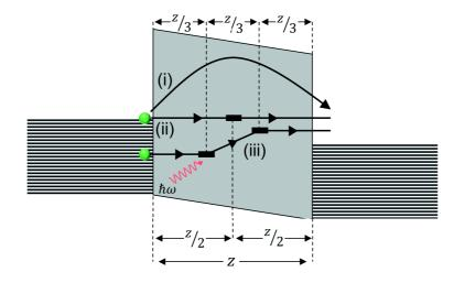
Figure 2.20: **Different tunneling path induced by localized states:** Paths (i), (ii) and (iii) repsectively represent direct tunneling, resonant tunneling through a single localized states (LS) and inelastic hopping through a chain of two LS. The red arrow represents the absorption of a phonon during the hopping. Adapted from Xu *et al.*<sup>148</sup>.
