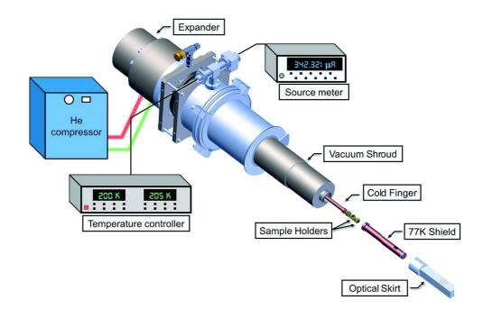
Figure 3.6: **4K Gifford-McMahon cryostat:** Standard magnetotransport bench composed of a cryostat, a temperature controller, a source meter, two magnets (not shown) and a computer with a LabView control program (not shown). Other elements such as an electrical multiplex transmitter, motors, optical tables and optical elements are not shown.
