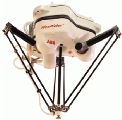
(b) Robot parallèle FlexPicker d'ABB Automation and Power Technologies
