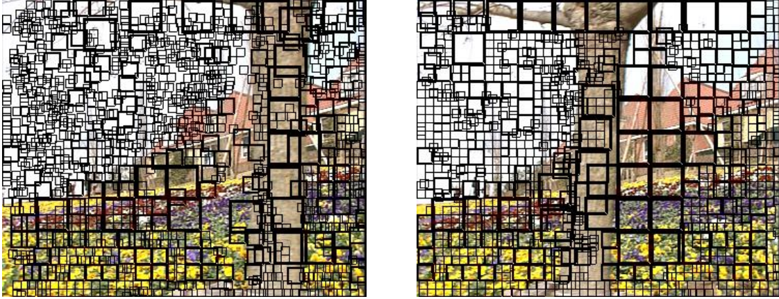
Figure 37: Trajectories grouping for Flower CIF sequence, for frames 200 and 218, using original square sections of size 8.
