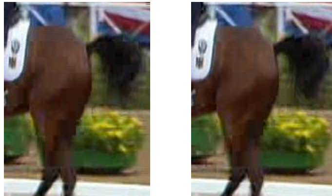
Figure 61: Part of decoded frame with uniform QP (left) and with locally adapted QP with proposed method (right).
