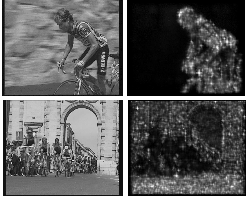
Figure 57: Original (left) and corresponding quality maps (right) (higher luminance means higher visibility).
