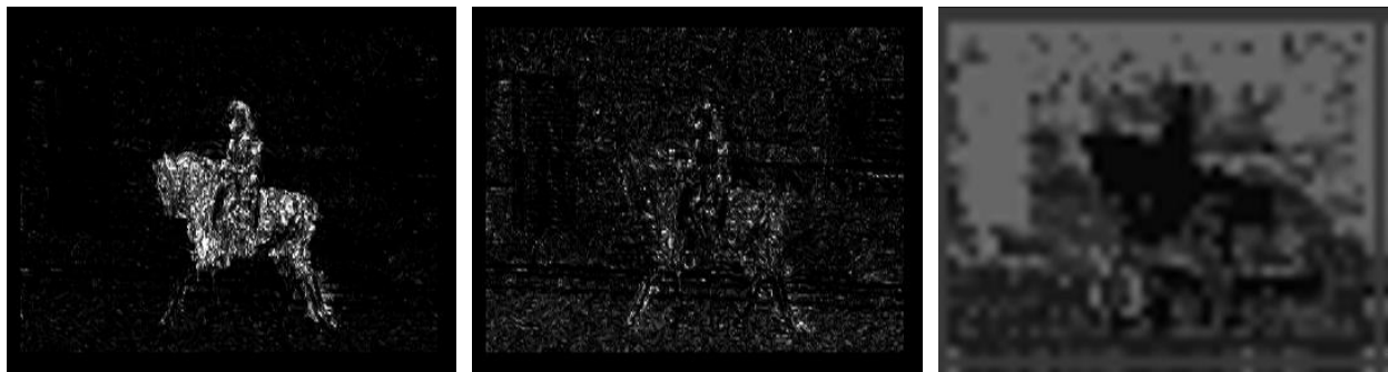
Figure 60: Quality-map at first iteration (left), quality-map at last iteration (center), QPs last iteration (right).
