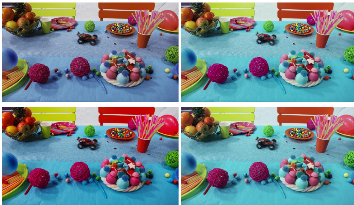
Figure 108: BT2020 graded (top-left), BT709 graded (top-right), BT2020 colour space conversion to BT709 (bot-left), BT2020 colour remapped with CRI (bot-right).
