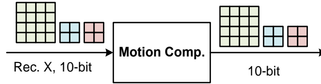
Figure 98: intra-layer temporal prediction (motion compensation) workflow process.
