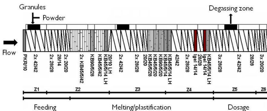
Figure 13: Screw profile used, where: 42/42, 28/28, 20/20 are right-handed screw elements; 20/10 LH is a left-handed screw element; KB 45/5/14, KB 45/5/28, KB 45/5/42, KB 90/5/20, KB 90/5/28 are right-handed kneading disc blocks; KB 45/5/14 LH is a left-handed kneading disc block; Igel 14/14 is a mixing element type "turbine".
