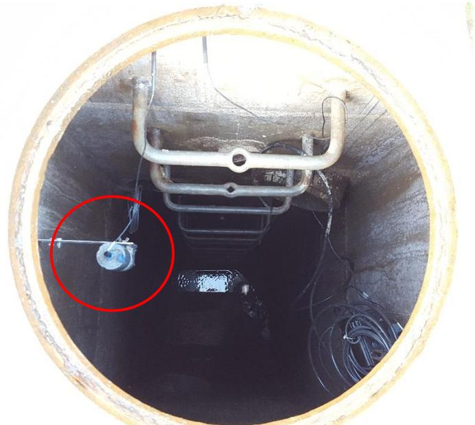
Figure 2-22: Water Depth Meter installed in the last manhole of the Studied Sector
