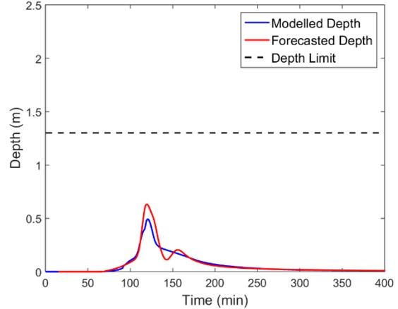
Figure 4-19: Modelled and Forecasted Water Depth at Critical Manhole 2 – 1 YRP Event
