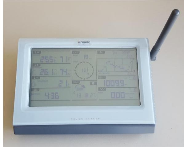
*Figure 2-18: Display/Receiver Console*
