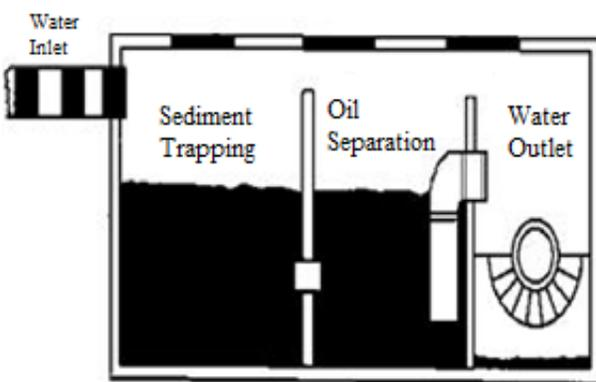
Figure 1-14: Oil and sediment separator (Schueler 1987)
