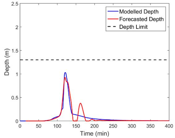
Figure 4-17: Modelled and Forecasted Water Depth at Critical Manhole 1 – 2 YRP Event
