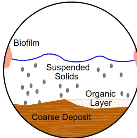
Figure 1-3: Different layers of solid deposits in networks
