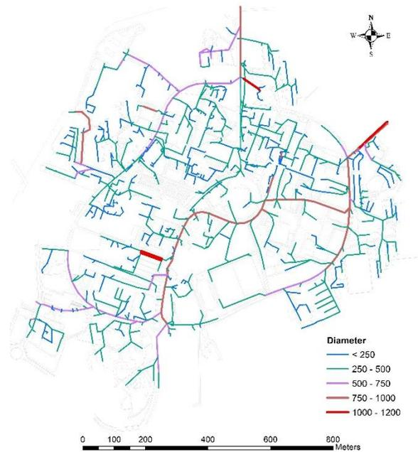
Figure 2-5: Diameter of Stormwater network pipes digitized within the GIS Layers
