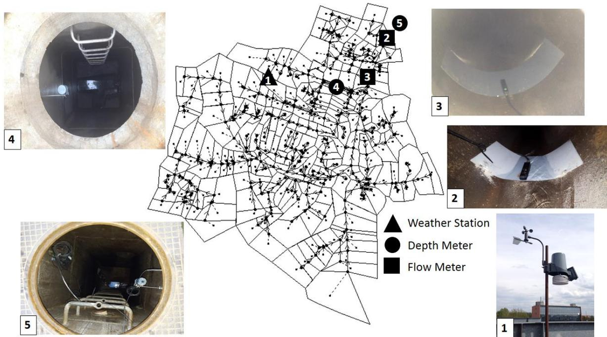
Figure 3-2: Urban Drainage System within the Studied Sector and the Implemented Quantitative Sensors
