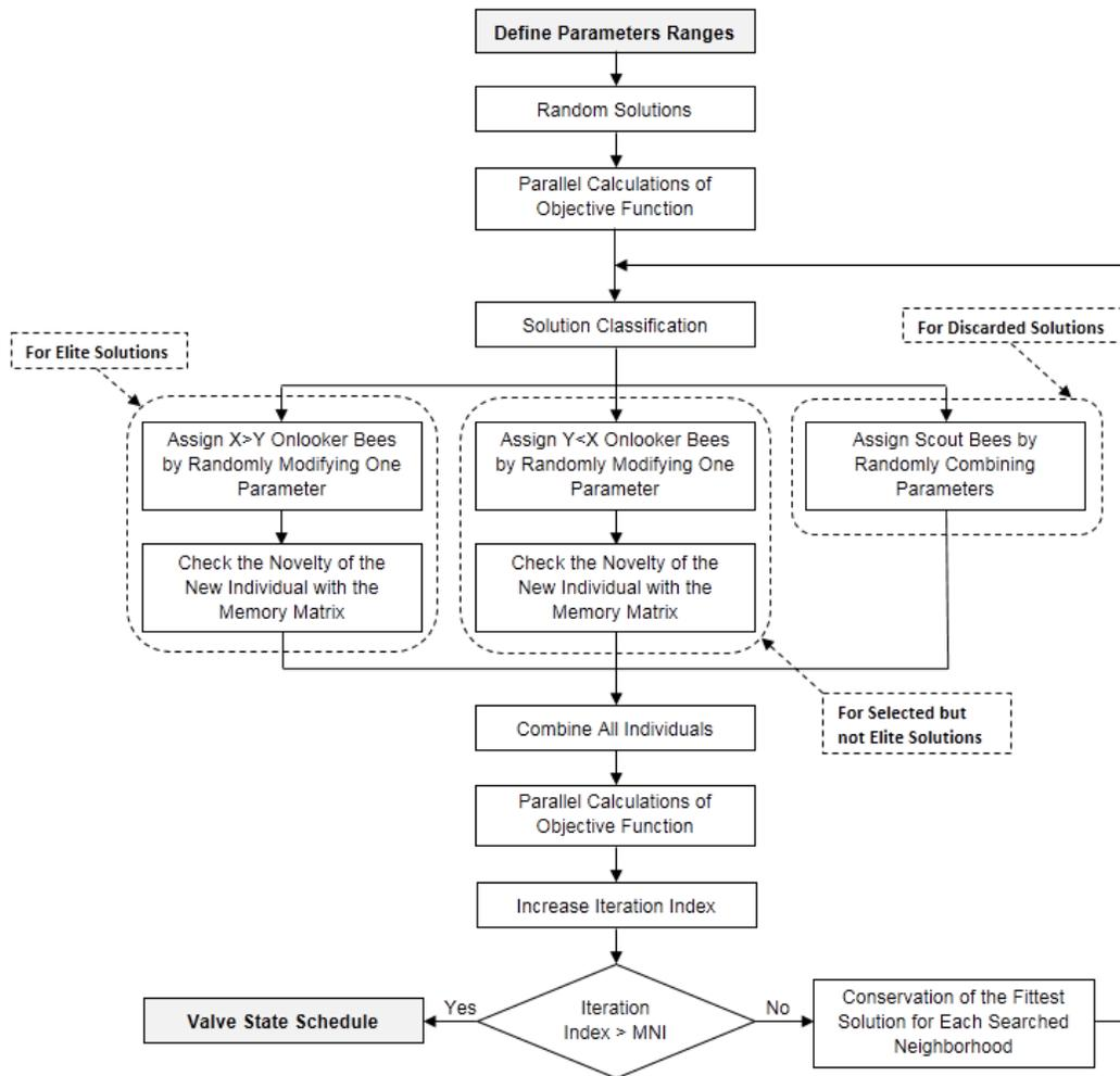
Figure 4-32: Calculation Steps of the Modified Artificial Bee Colony
