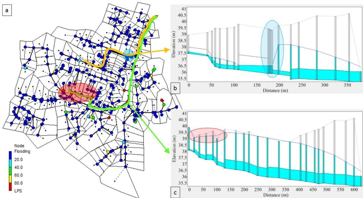
Figure 4-1: Model Results for the Storm Event of 31 August 2015 - 14:09 (a-Plan View Showing the Flooding Areas b-Profile Plot through the Retention Tank c-Profile Plot through the Flooding Areas)
