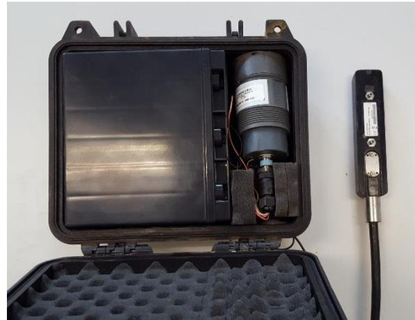
Figure 2-28: Flowmeter with Rechargeable Battery Pack Installed Downstream the Retention Tank
