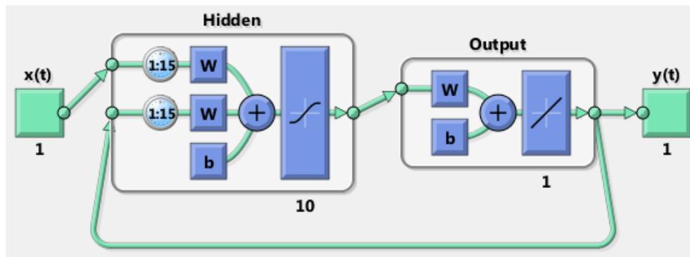
Figure 3-23: NARX Neural Network for Forecasting Downstream Boundary Conditions of the EPA-SWMM Model
