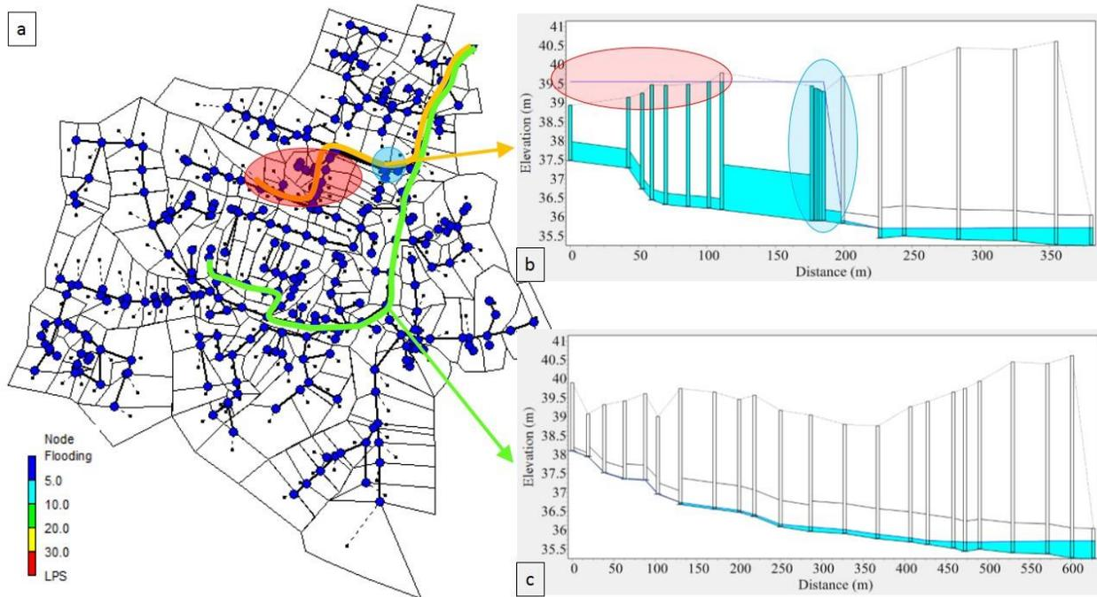
Figure 4-11: Model Results for the 5 Year Return Period Synthetic Storm Event – 3:03 (a-Plan View of the System b-Profile Plot through the Retention Tank c-Profile Plot through the Principal Collector)
