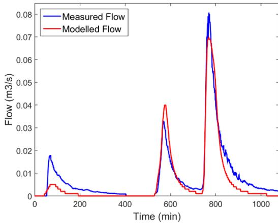
Figure 3-11: Measured and Modelled Flow Comparison for Rainfall Event 28/10/2015 (NSE=0.91)
