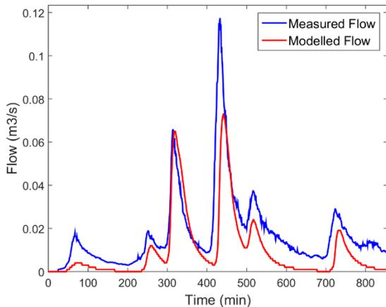
Figure 3-7: Measured and Modelled Flow Comparison for Rainfall Event 24/08/2015 (NSE=0.47)
