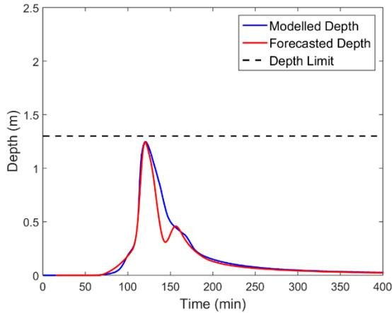
Figure 4-28: Modelled and Forecasted Water Depth at Critical Manhole 5 – 1 YRP Event
