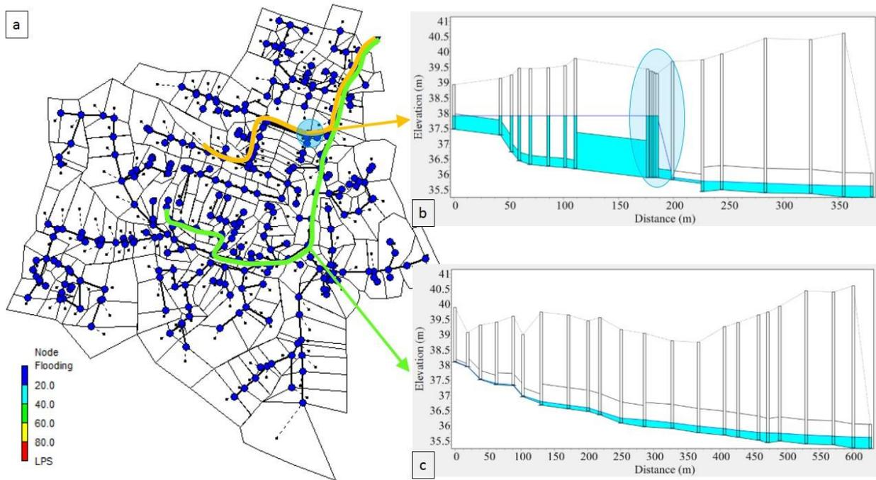
Figure 4-3: Model Results for the Storm Event of 31 August 2015 - 15:11 (a-Plan View of the System b-Profile Plot through the Retention Tank c-Profile Plot through the Principal Collector)
