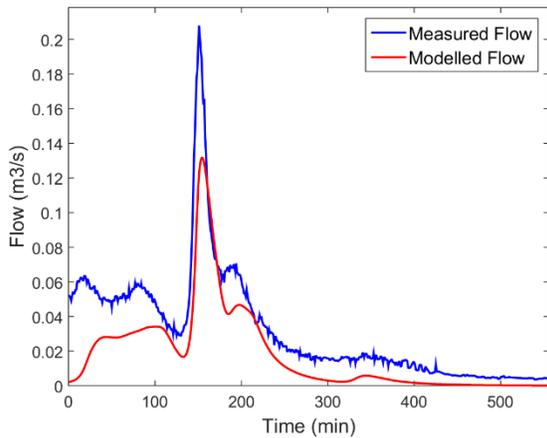
Figure 3-13: Measured and Modelled Flow Comparison for Rainfall Event 27/08/2015 (NSE=0.62)
