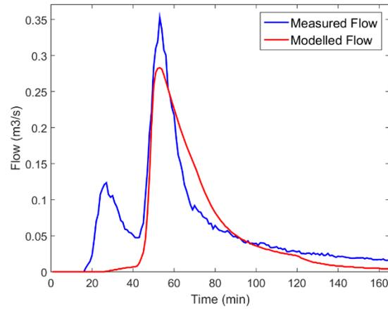
Figure 3-6: Measured and Modelled Flow Comparison for Rainfall Event 04/08/2015 (NSE=0.74)
