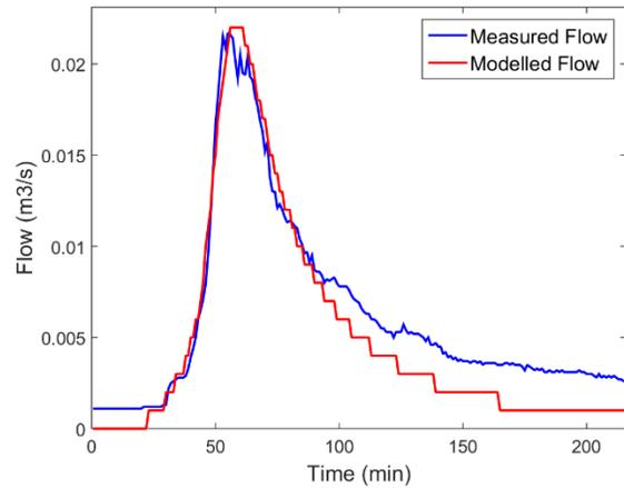
Figure 3-12: Measured and Modelled Flow Comparison for Rainfall Event 07/11/2015 (NSE=0.90)
