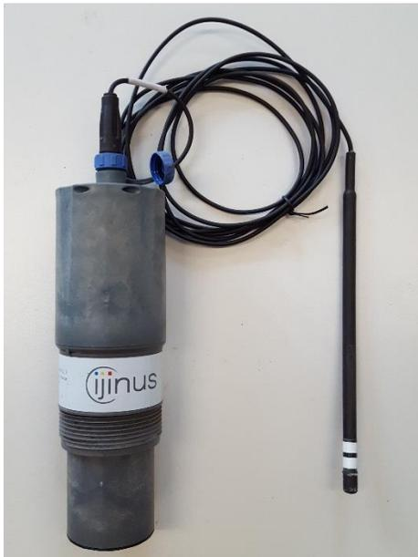
Figure 2-21: Water Depth Meter with a measuring range 0.3 to 6 m
