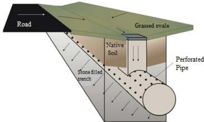
Figure 1-13: Drainage system using perforated pipes to increase soil infiltration (Jun 2010)
