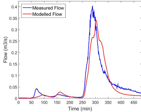
Figure 3-4: Measured and Modelled Flow Comparison for Rainfall Event 25/07/2015 (NSE=0.82)
