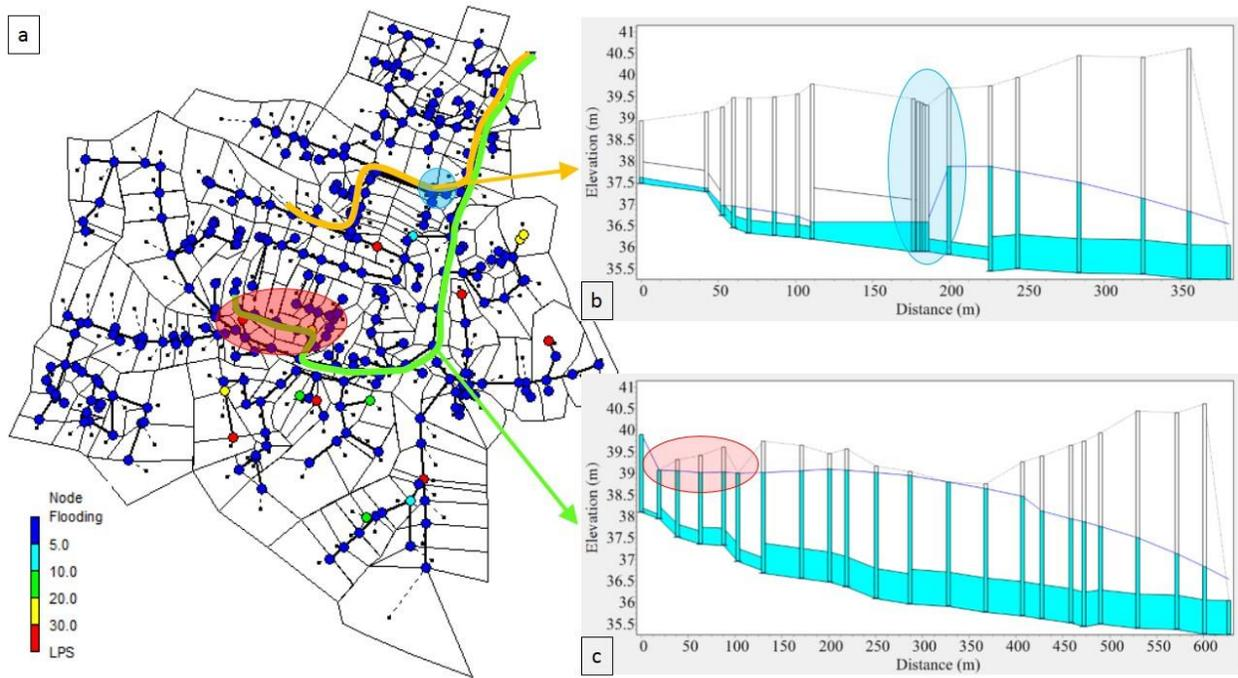
Figure 4-10: Model Results for the 5 Year Return Period Synthetic Storm Event – 1:03 (a-Plan View of the System b-Profile Plot through the Retention Tank c-Profile Plot through the Principal Collector)
