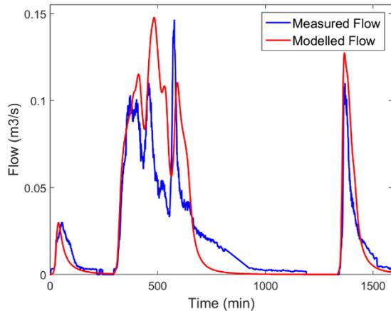
Figure 3-21: Measured and Modelled Flow Comparison for Rainfall Event 09/02/2016 ( $NSE=0.53$ )
