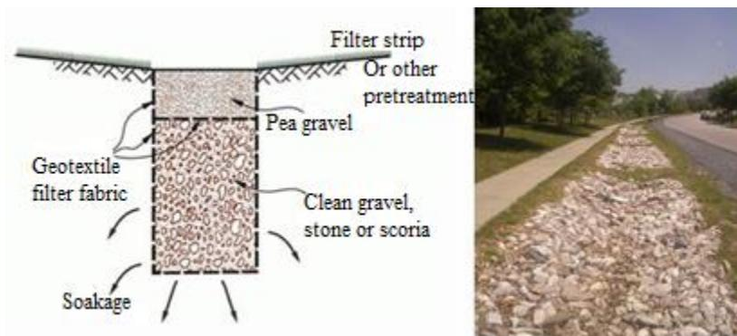
Figure 1-6: Drainage Trench (RiverSides ; Sustainable Stormwater Management 2007)
