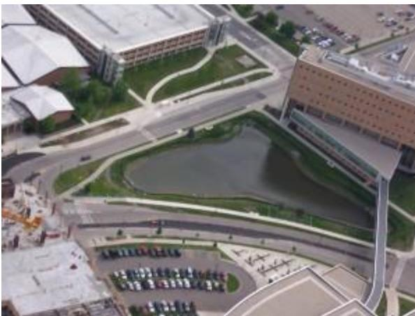
Figure 1-8: Retention or detention pond (Strand Associates 2011)
