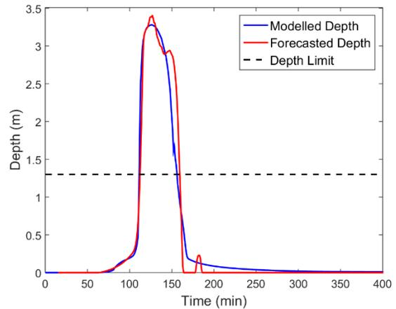
Figure 4-21: Modelled and Forecasted Water Depth at Critical Manhole 2 – 5 YRP Event
