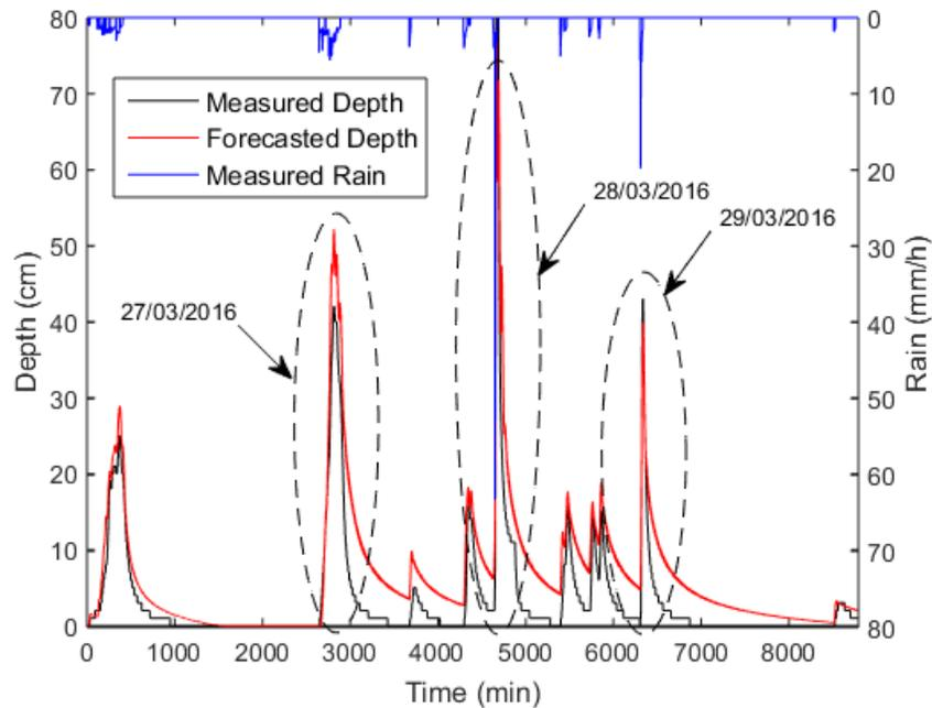
Figure 3-26: Comparison of Measured and Forecasted Outfall Water Depth for the Rainfall Events Occurring between 25 and 30 March 2016
