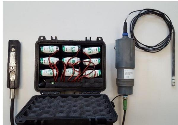
Figure 2-24: Flowmeter with Lithium Battery Pack, Installed at the Outfall of the Studied Sector
