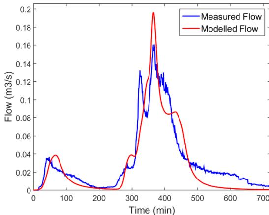
Figure 3-19: Measured and Modelled Flow Comparison for Rainfall Event 30/01/2016 (NSE=0.81)
