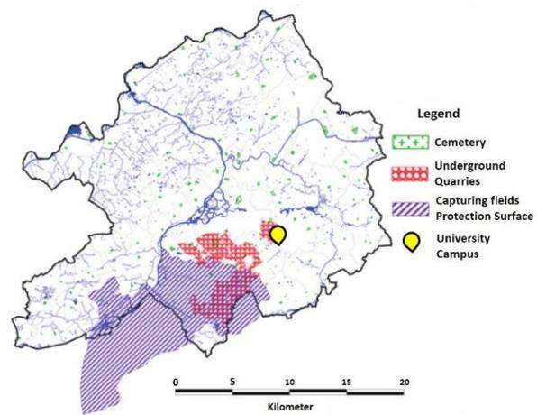
Figure 2-40: Regulatory Constraints Limiting the Infiltration Applicability
