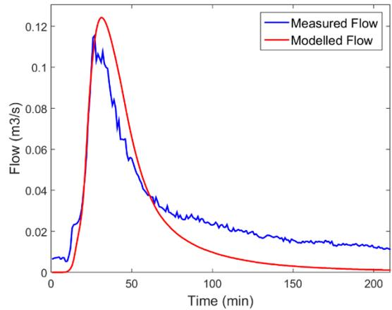
Figure 3-30: Measured and Modelled Flow Comparison for Rainfall Event 29/03/2016 (NSE=0.73)
