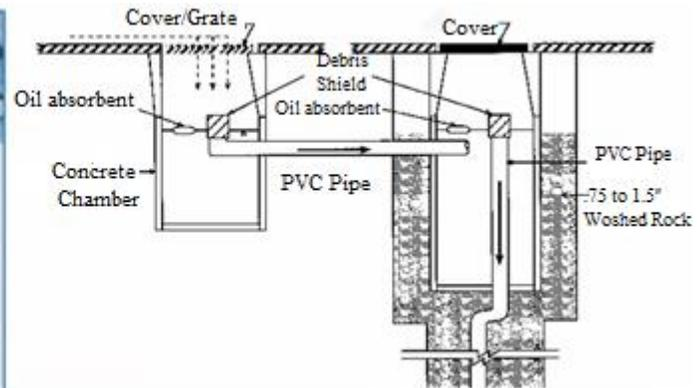
Figure 1-12: Infiltration well (US EPA 2013) & (GUIDEnR HQE)
