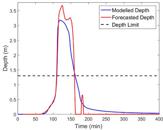
Figure 4-30: Modelled and Forecasted Water Depth at Critical Manhole 5 – 5 YRP Event
