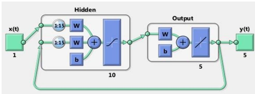
Figure 4-13: NARX Neural Network for Forecasting Flooding Events
