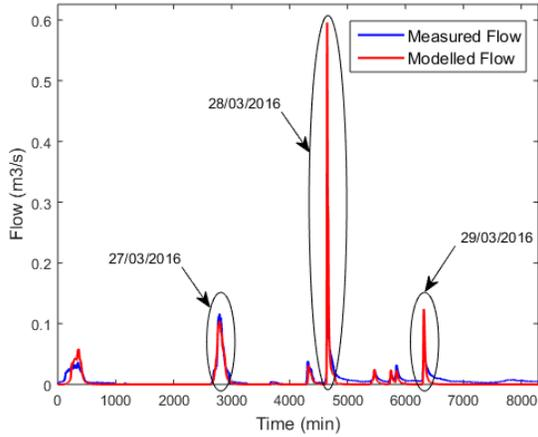
Figure 3-27: Measured and Modelled Flow Comparison (Rainfall Events 25-30/03/2016)
