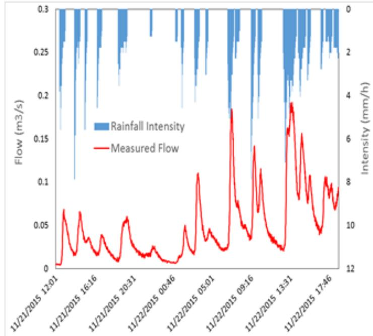
Figure 2-16: Rainfall Intensity and Flow Measurements in 22 November 2015 Storm Event
