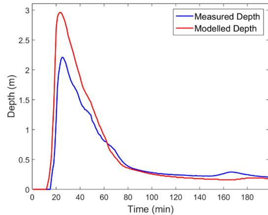
Figure 3-14: Measured and Modelled Flow Comparison for Rainfall Event 31/08/2015 (NSE=0.73)
