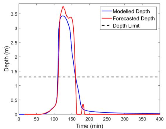
Figure 4-27: Modelled and Forecasted Water Depth at Critical Manhole 4 – 5 YRP Event
