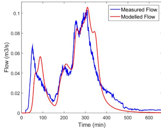
Figure 3-22: Measured and Modelled Flow Comparison for Rainfall Event 04/03/2016 ( $NSE=0.79$ )
