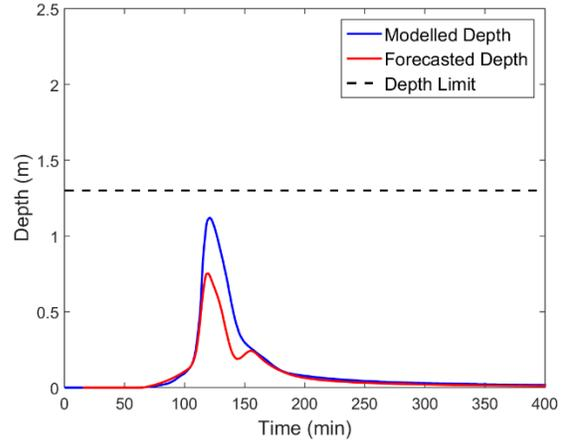
Figure 4-25: Modelled and Forecasted Water Depth at Critical Manhole 4 – 1 YRP Event
