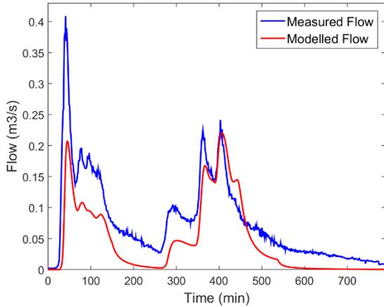
Figure 3-15: Measured and Modelled Flow Comparison for Rainfall Event 19/11/2015 (NSE=0.52)
