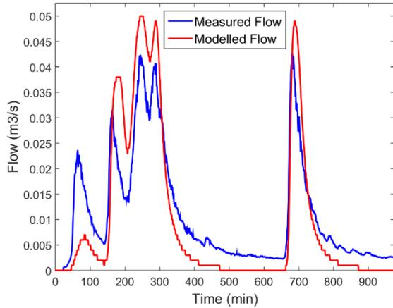
Figure 3-3: Measured and Modelled Flow Comparison for Rainfall Event 14/05/2015 (NSE=0.64)
