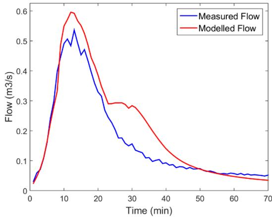
Figure 3-29: Measured and Modelled Flow Comparison for Rainfall Event 28/03/2016 (NSE=0.82)
