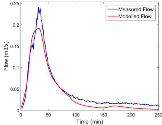
Figure 3-18: Measured and Modelled Flow Comparison for Rainfall Event 11/12/2015 (NSE=0.95)
