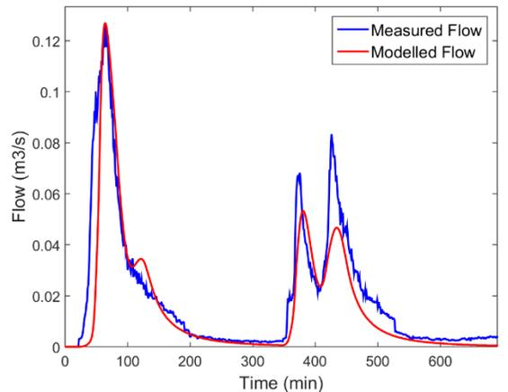
Figure 3-20: Measured and Modelled Flow Comparison for Rainfall Event 08/02/2016 (NSE=0.79)
