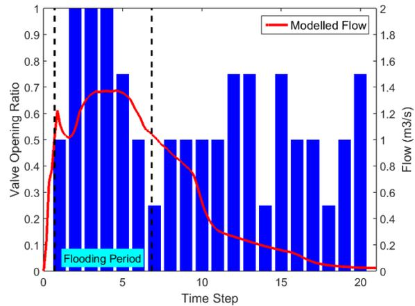
Figure 4-63: Flow in the Main Collector and Optimal VSS for the Event of 31 August 2015
