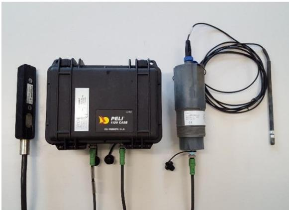
Figure 2-23: Different Parts of the Flowmeter Installed at the Outfall of the Sector (Probe, Battery, Transmitter)
