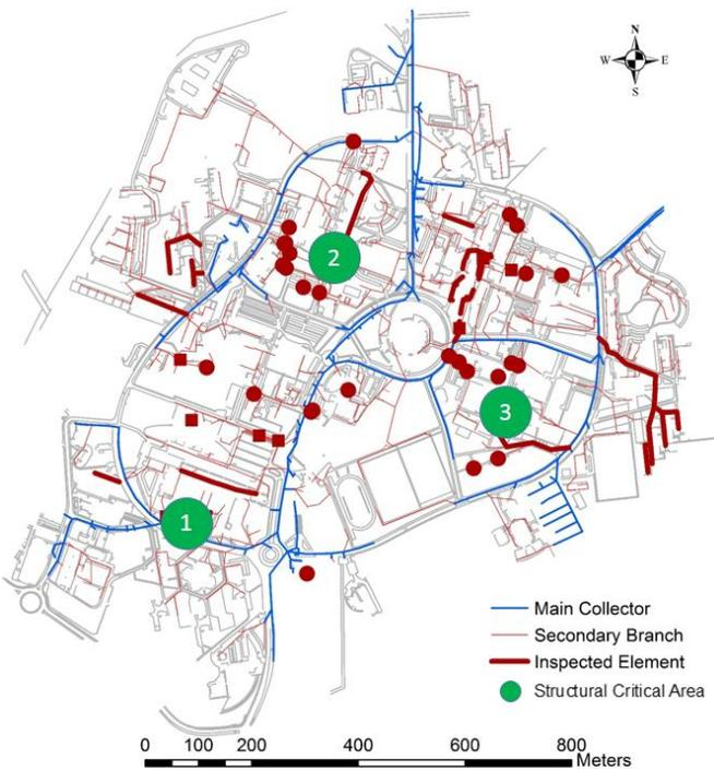
Figure 2-9: Structural Critical Areas within the UDS of the Campus
