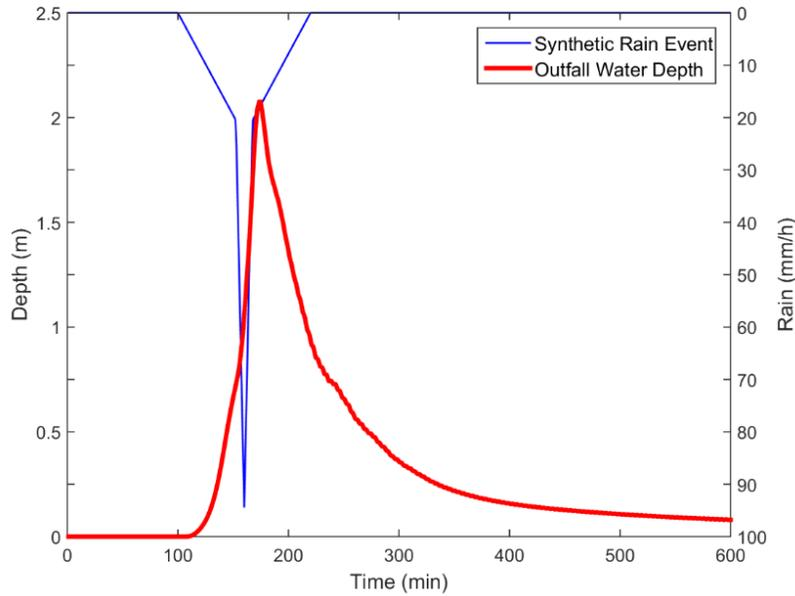
Figure 4-7: Outfall Water Depth for the Event of 5 Year Return Period, Calculated by NARX Neural Network
