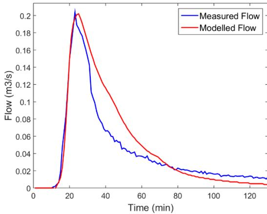
Figure 3-5: Measured and Modelled Flow Comparison for Rainfall Event 30/07/2015 (NSE=0.84)
