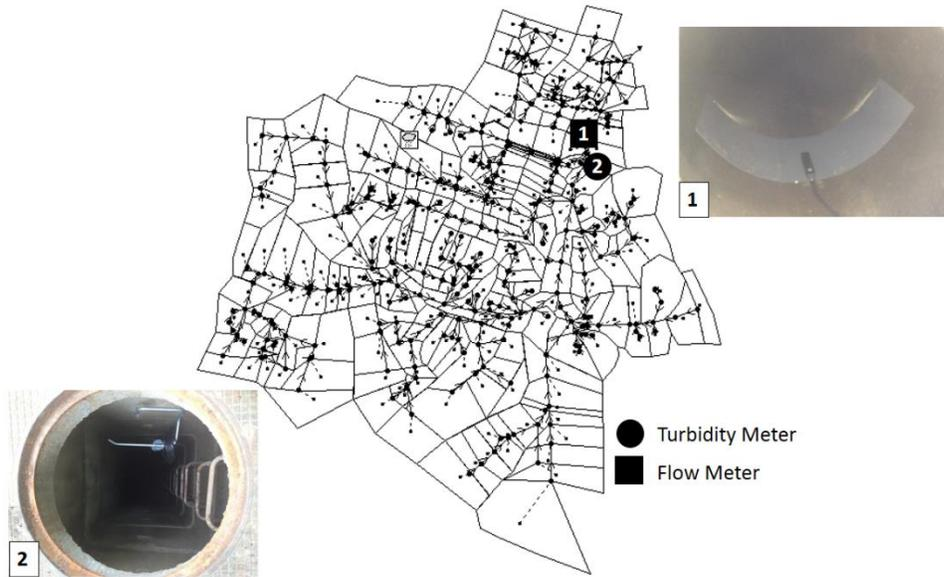
Figure 4-66: Flowmeter and Turbidity Meter Implemented on the Lille 1 University Campus
