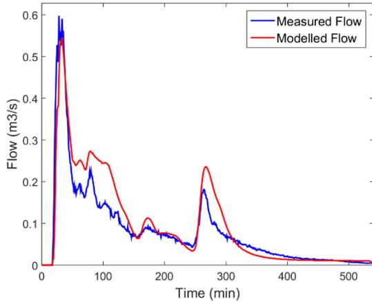
Figure 3-9: Measured and Modelled Flow Comparison for Rainfall Event 13/09/2015 (NSE=0.82)
