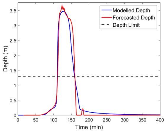
Figure 4-24: Modelled and Forecasted Water Depth at Critical Manhole 3 – 5 YRP Event
