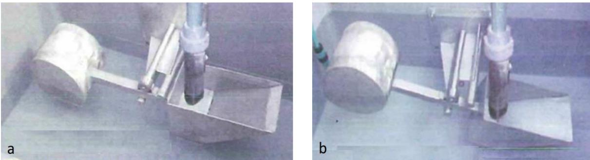
Figure 1-17: In-line Turbidity Meter Installation (a-Submerged Probe during Low Water Level b-Real Time Measurements during Rainfall Events)
