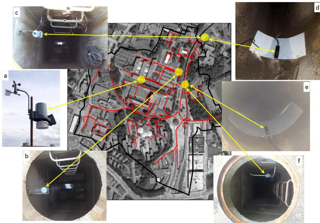
Figure 2-15: Monitoring System Installed on the Studied Sector of Lille 1 University Campus
