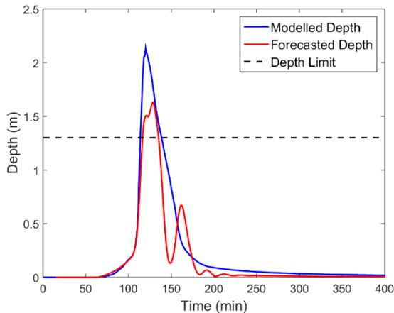
Figure 4-26: Modelled and Forecasted Water Depth at Critical Manhole 4 – 2 YRP Event
