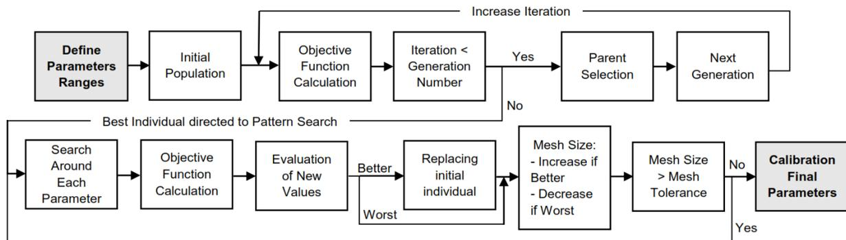
Figure 3-1: Auto-Calibration Process based on Genetic Algorithm and Pattern Search
