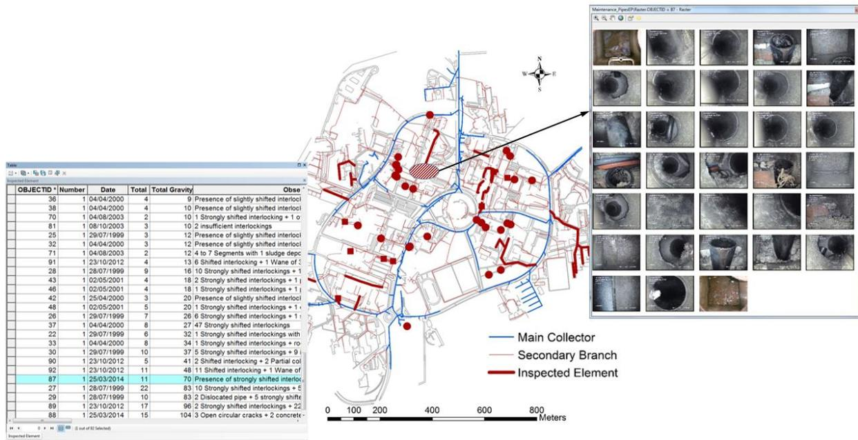
Figure 2-7: Inspection Layer within the GIS Database, with an Example of Observations taken from an Inspected Pipe
