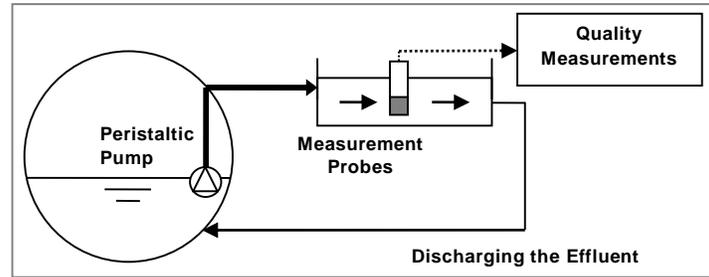
Figure 1-18: Illustration of Parallel Real Time Measurement By-Pass Chamber
