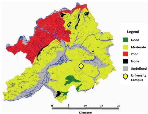
Figure 2-39: Infiltration Potential Based on Soil Type and Thickness of Unsaturated Layer
