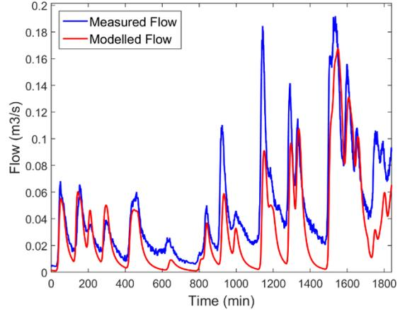
Figure 3-16: Measured and Modelled Flow Comparison for Rainfall Event 21/11/2015 (NSE=0.60)
