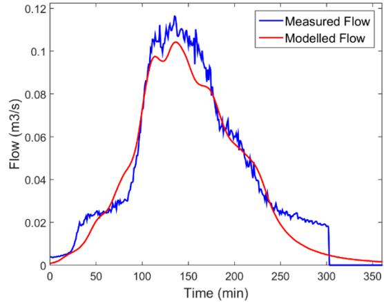
Figure 3-28: Measured and Modelled Flow Comparison for Rainfall Event 27/03/2016 (NSE=0.96)
