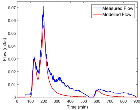
Figure 3-17: Measured and Modelled Flow Comparison for Rainfall Event 26/11/2015 (NSE=0.82)
