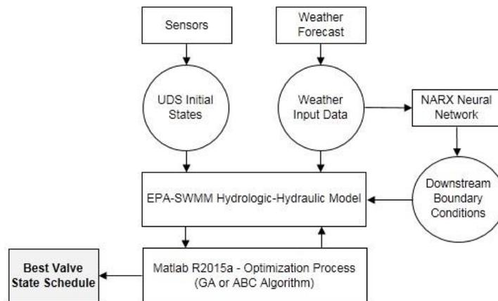
Figure 4-31: Valve State Schedule Optimization Process
