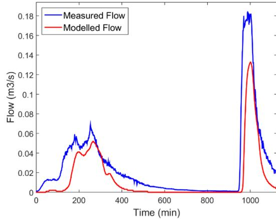
Figure 3-10: Measured and Modelled Flow Comparison for Rainfall Event 05/10/2015 (NSE=0.65)
