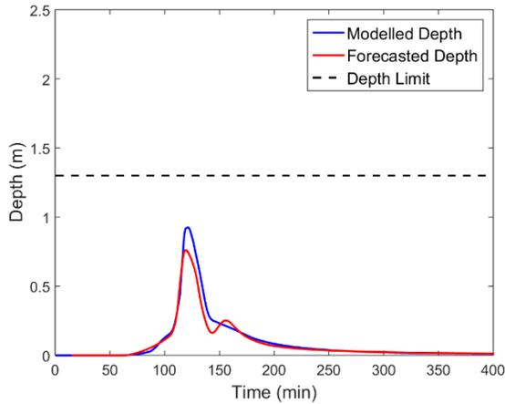
Figure 4-22: Modelled and Forecasted Water Depth at Critical Manhole 3 – 1 YRP Event
