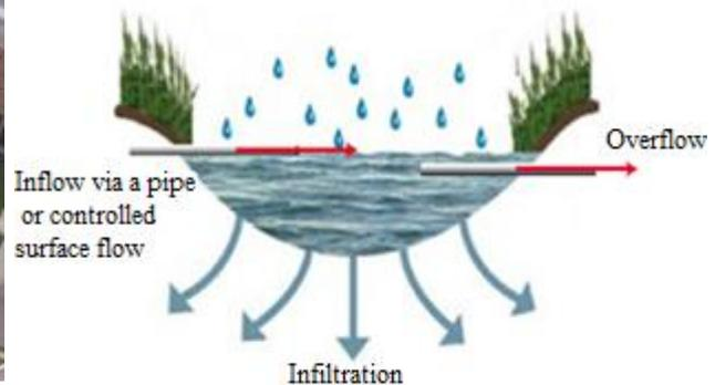
Figure 1-9: Infiltration basin (Vermont)
