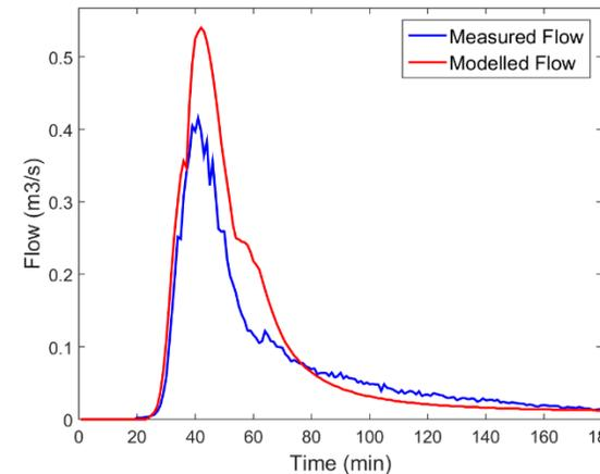
Figure 3-8: Measured and Modelled Flow Comparison for Rainfall Event 26/08/2015 (NSE=0.75)
