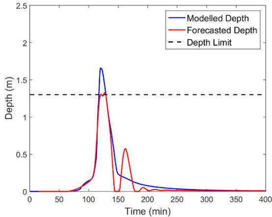
Figure 4-20: Modelled and Forecasted Water Depth at Critical Manhole 2 – 2 YRP Event
