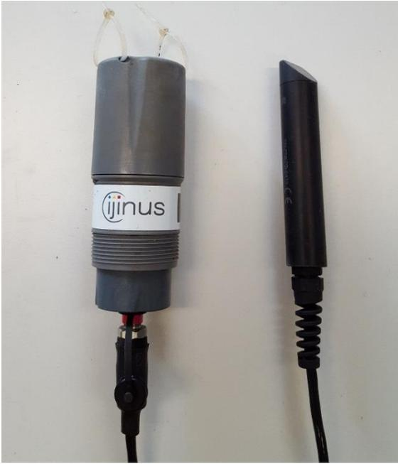
Figure 2-31: Data Logger and Probe of the Turbidity Meter
