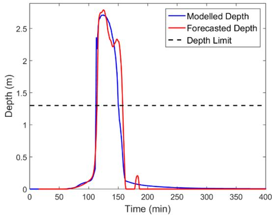
Figure 4-18: Modelled and Forecasted Water Depth at Critical Manhole 1 – 5 YRP Event
