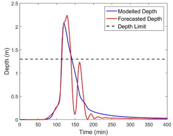
Figure 4-29: Modelled and Forecasted Water Depth at Critical Manhole 5 – 2 YRP Event
