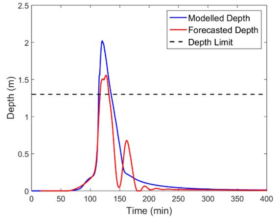
Figure 4-23: Modelled and Forecasted Water Depth at Critical Manhole 3 – 2 YRP Event
