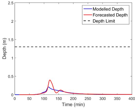
Figure 4-16: Modelled and Forecasted Water Depth at Critical Manhole 1 – 1 YRP Event
