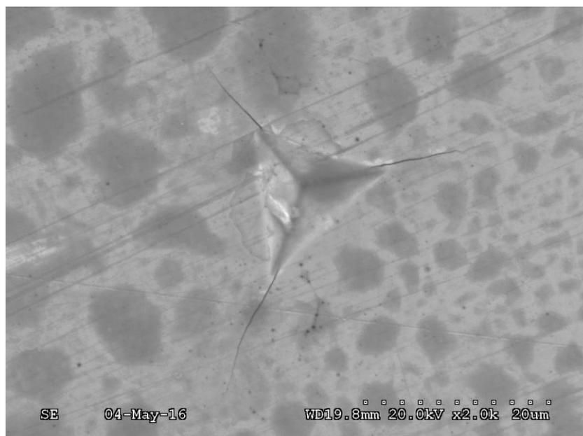
Figure III.3-9. SEM micrograph from the residual impression from a Berkovich indenter on the sample labeled as 1020-I after standard indentation test with a maximum applied load 1 N is accomplished.
