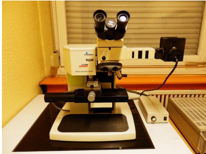
Figure II.3-1. Microhardness indenter CSM 2–107 manufactured by CSM instruments used to perform the instrumented indentation tests at the microscale range.
