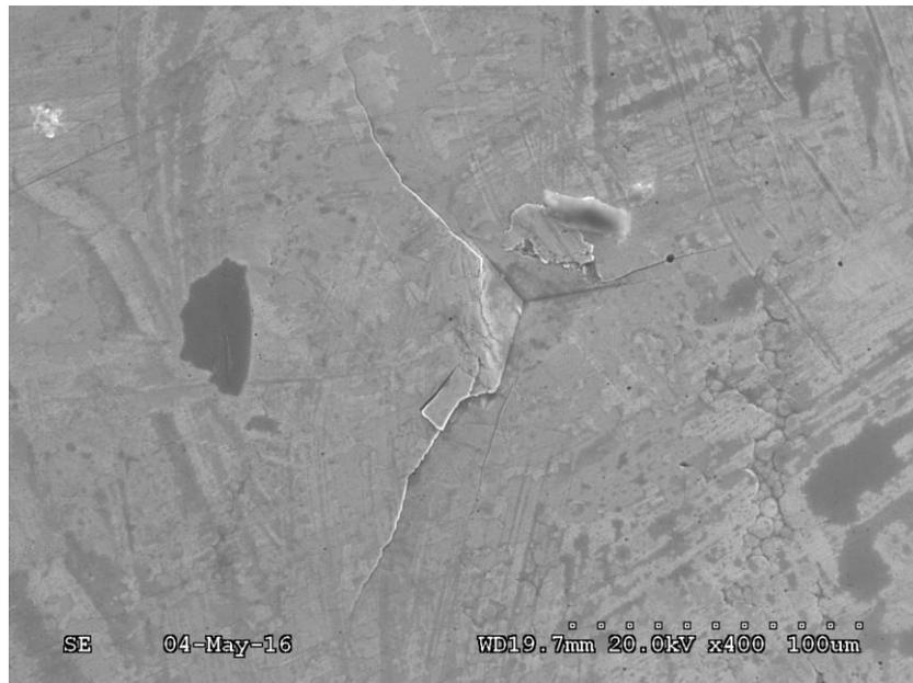
Figure III.3-10. SEM micrograph from the residual impression from a Berkovich indenter on the sample labeled as 1020-I after standard indentation test with a maximum applied load 18 N is effected.
