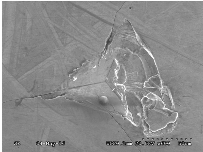
Figure III.3-8. SEM micrograph from the residual impression from a Berkovich indenter on the sample labeled as 1020-I after a continuous multicycle indentation test of 100 cycles is accomplished.
