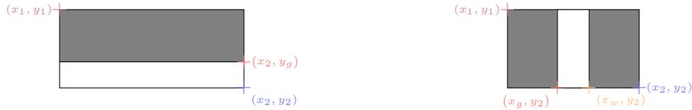
FIGURE 3.1: Example of Haar-like features used in Viola-Jones for face detection. They can be seen as convolution kernels where the grey parts correspond to  $+1$  coefficients, and the white ones  $-1$ . Such features can be computed efficiently using integral images [30, 136]. Point coordinates are presented here for latter use in the equations characterizing feature computations.
