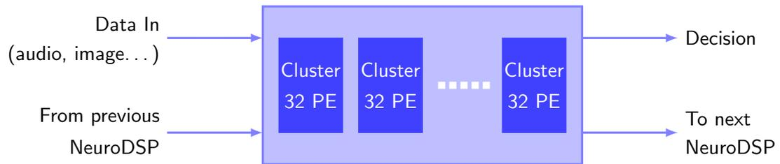
FIGURE 1.3: NeuroDSP architecture [5]. A NeuroDSP device is composed of 32 clusters, called *P-Neuro*, each constituted of 32 artificial neurons called PE, thus representing a total of 1024 neurons. The PEs may be multiplexed, so that they can perform several instructions sequentially and thus emulate bigger neural networks. When timing is critical, one may instead cascade several NeuroDSP processors and use them as if it was a single device.
