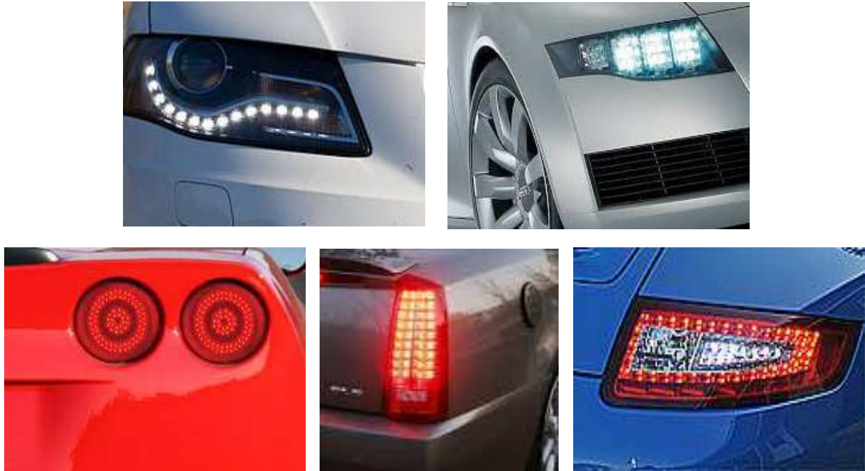
Figure 2.2: Integration of LEDs lighting systems in series vehicles – processed using [94].
