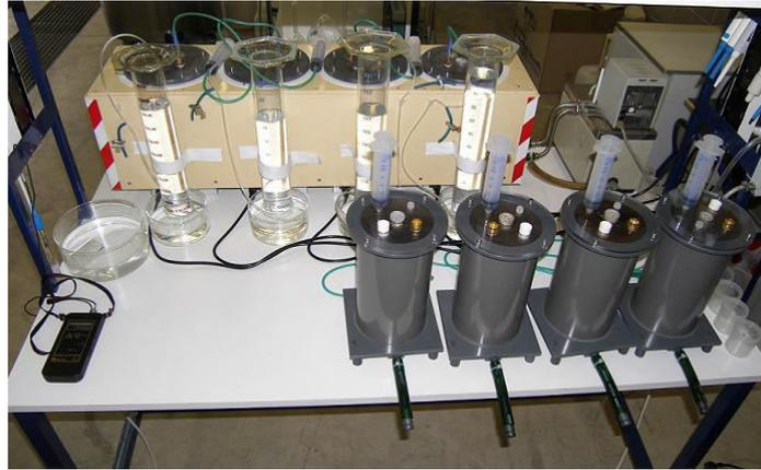
Figure 1: Photo of pilot plan with 8 aerobic and anaerobic reactors.
