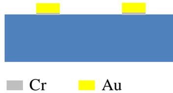
**Figure 2.8: Metallic patterns deposited on the surface of the substrate.**
