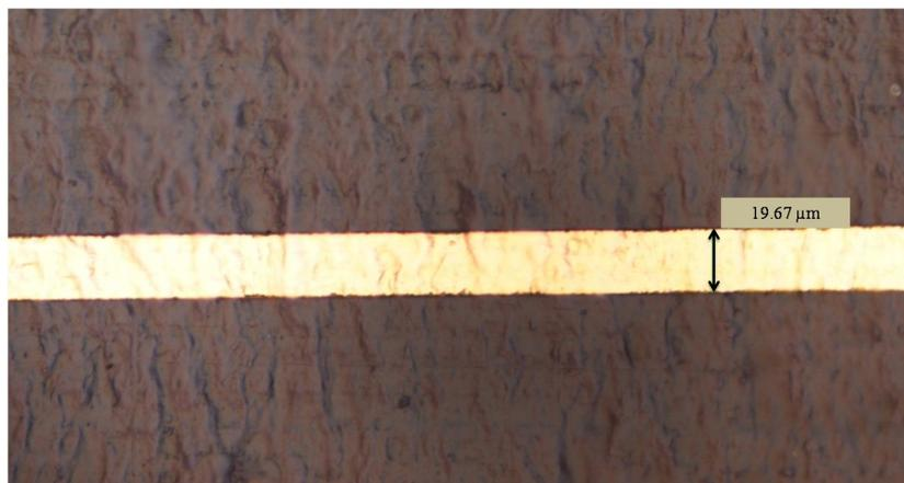
Figure 4.5: A metallic line of 20  $\mu\text{m}$  width prepared by photolithography.
