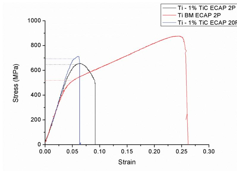
Figure 88: Compression test of Ti -1% TiC ECAPed for 2 passes (black) compared to Ti BM (red) – (the curves are not corrected from the equipment rigidity making the E value not accurate)
