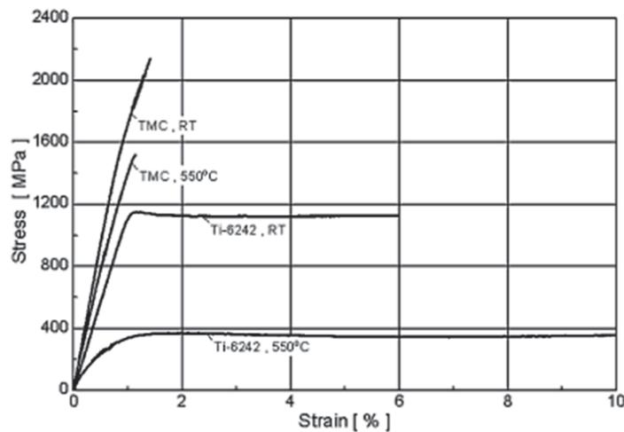
Figure 9: Stress-strain for Ti-62642 (near α) and the TMC Ti-62642/SiC fibres 35%vol. [BET2007]
