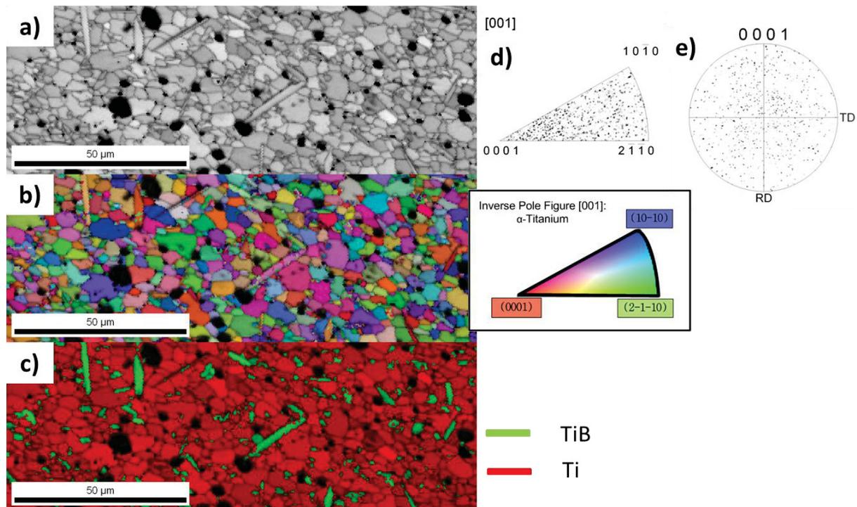
Figure 92: EBSD analysis of Ti - 10% TiB sample (pressureless sintering) with a) SEM micrograph, b) grain orientation, c) phases, d) inverse pole figure for Ti and e) pole figure for Ti (step size 0.50 μm, map size: 140 μm / 50 μm)
