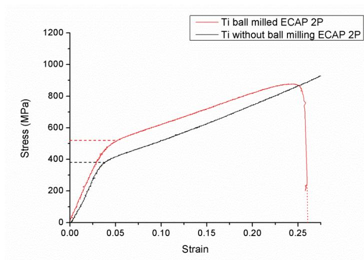
**Figure 82: Compression test of Ti ECAPed for 2 passes, without ball milling (black) and with ball milling (red) – (the curves are not corrected from the equipment rigidity making the E value not accurate)**
