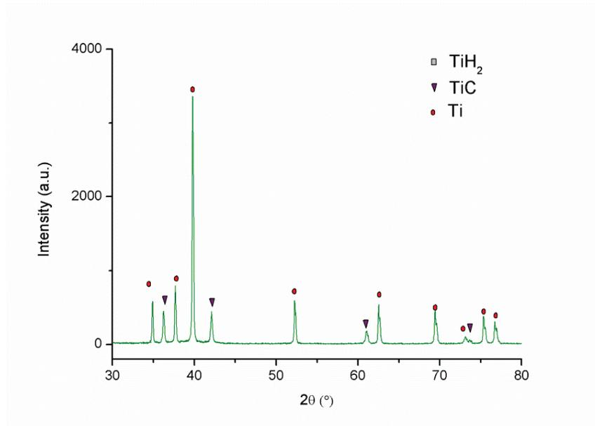
Figure 95: XRD spectrum of Ti - 10% TiC hot pressed at 800°C for 30 minutes
