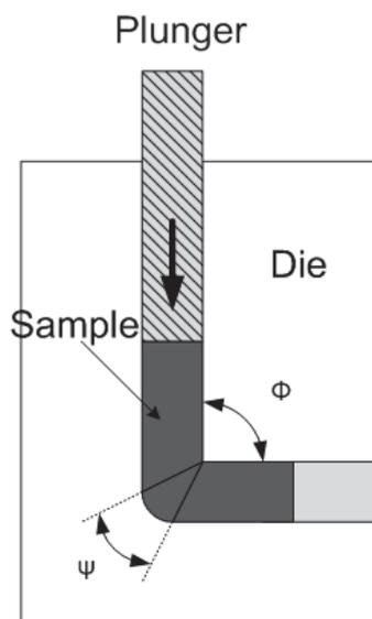
Figure 24: Schematic drawing of an ECAP setup [IWA1997]
