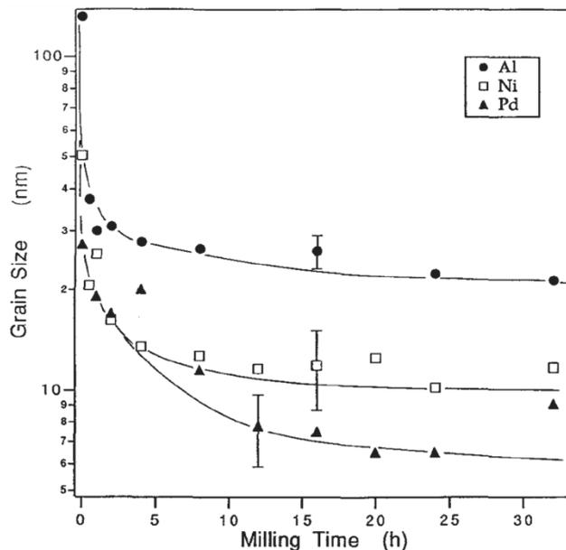
Figure 16: Average grain size evolution of Al, Ni and Pd powders depending on BM time [ECK1992]
