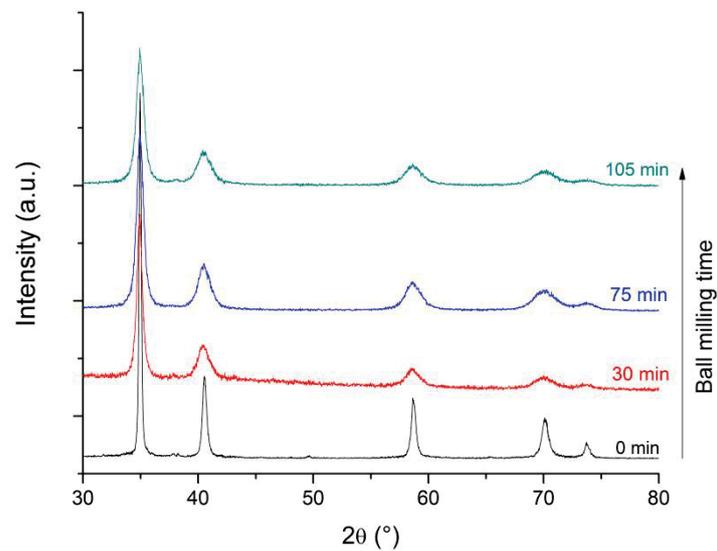
Figure 49: XRD spectra of TiH<sub>2</sub> powder at different ball milling times
