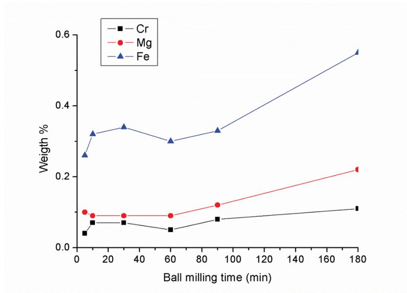
Figure 53: ICP analysis of  $\text{TiH}_2$  powder ball milled for different times (black: Cr, red: Mg, blue: Fe)
