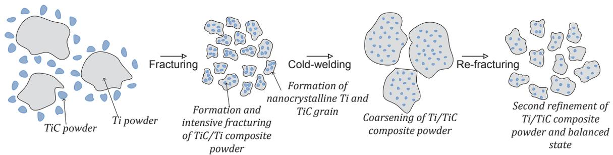
Figure 18: Schematic evolution of brittle-ductile Ti-TiC composite during BM [GU2010]
