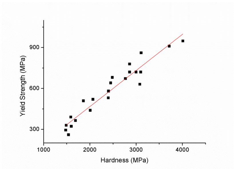
Figure 70: Yield Strength vs Hardness for several Ti based materials [REF-FIG70]
