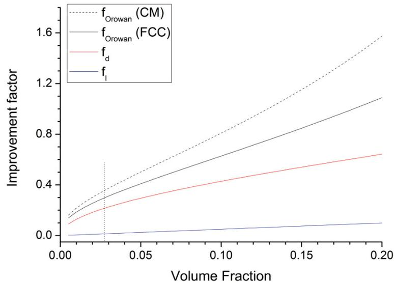
Figure 43: Improvement factors versus volume fraction of TiC in a Ti/TiC (40 nm) composite
