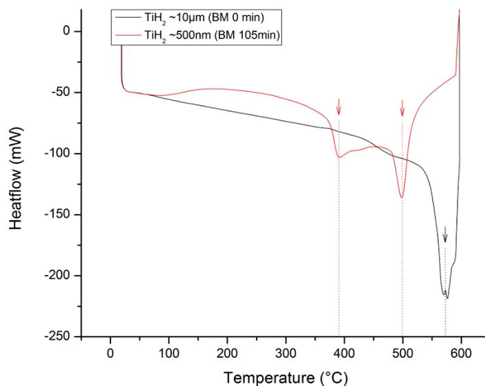
Figure 30: Evolution of the dehydrogenation temperature depending on the particle size
