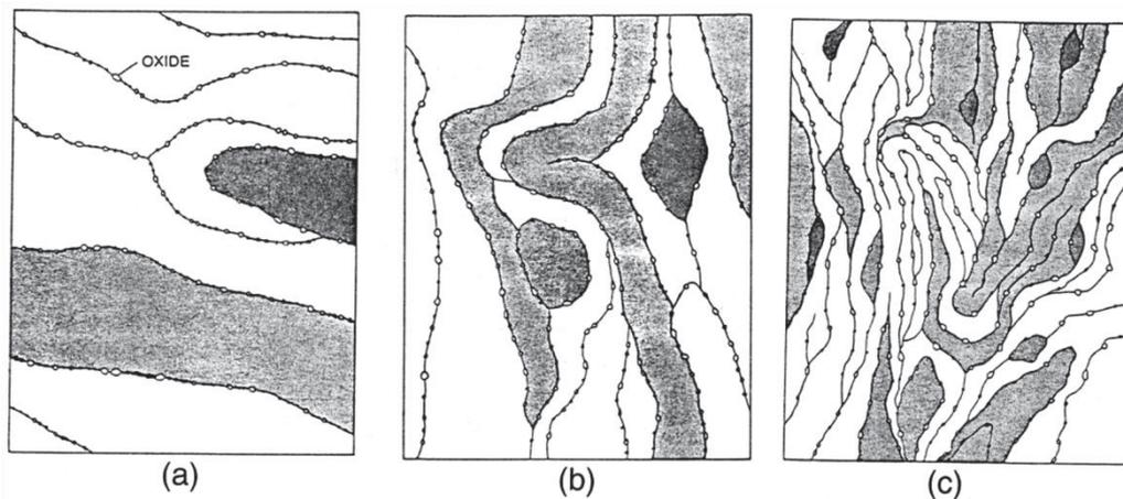
**Figure 17: Evolution of brittle-ductile powders during different stage of ball milling a) Early stage; Oxide is trapped between lamellar particles b) and c) Evolution of the system and dispersion of the brittle particles after longer time of BM [SUR2001]**
