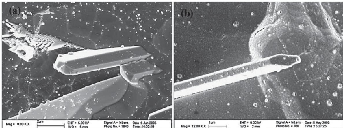
Figure 12: Typical shape of TiB whiskers in Ti matrix [LU2008]
