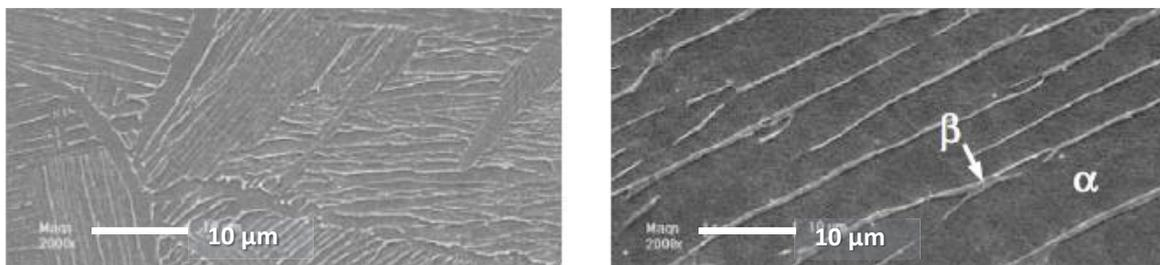
**Figure 5: Lamellar  $\alpha + \beta$  microstructure from the  $\beta$ -phase at a slow cooling rate. Air cooled on the left (slow) and furnace cooled on the right (very slow) [KIM2008]**
