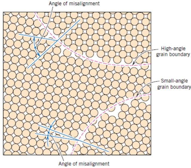
Figure 33: Schematic diagram of the LAGB and HAGB [CAL2007]
