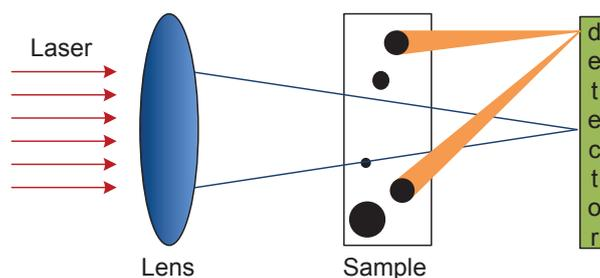
Figure 48: Schematic representation of the laser granulometry principle
