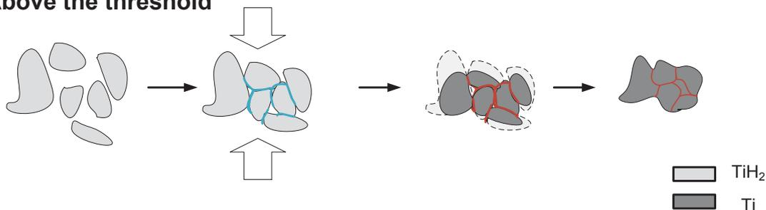
Figure 32: HDH sintering phenomena depending on the effect of the cold compaction
