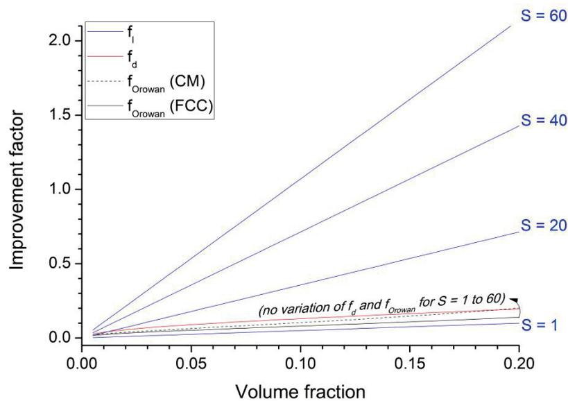
Figure 39: Improvement factor versus volume fraction for Ti/TiB<sub>w</sub> composite at different aspect ratio
