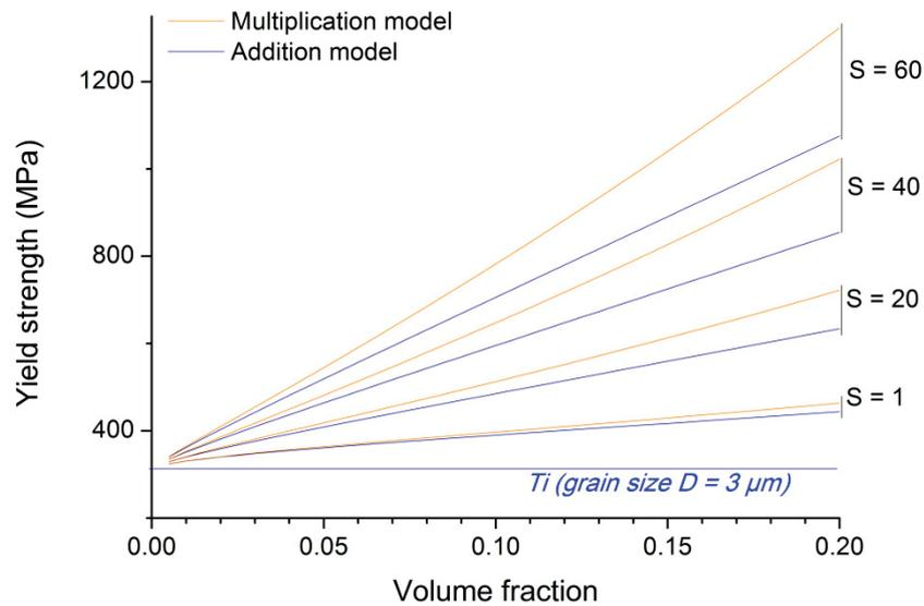
Figure 40: Yield strength versus volume fraction of  $TiB_w$  for the  $Ti/TiB_w$  composite at different aspect ratio
