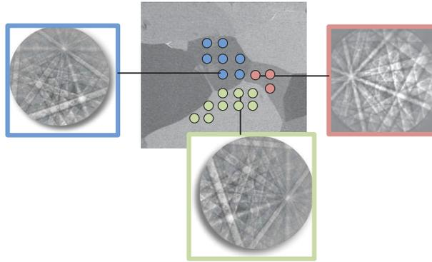
Figure 69: Example of the mapping during EBSD analysis
