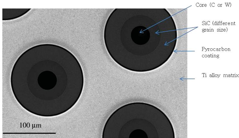
Figure 8: SEM-micrograph of Ti/SiC fibre composite [BET2007]
