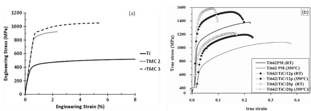
Figure 10: a) Engineering tensile test curves for cp-Ti (grade 2)/15%vol. TiC (2.6  $\mu\text{m}$ ) at room temperature [FRU2012] and b) Tensile test curves of a Ti-6Al-6V-2Sn reinforced with 12 and 20 vol.% of TiC particles (10  $\mu\text{m}$ ) at RT and 350°C [POL2012]
