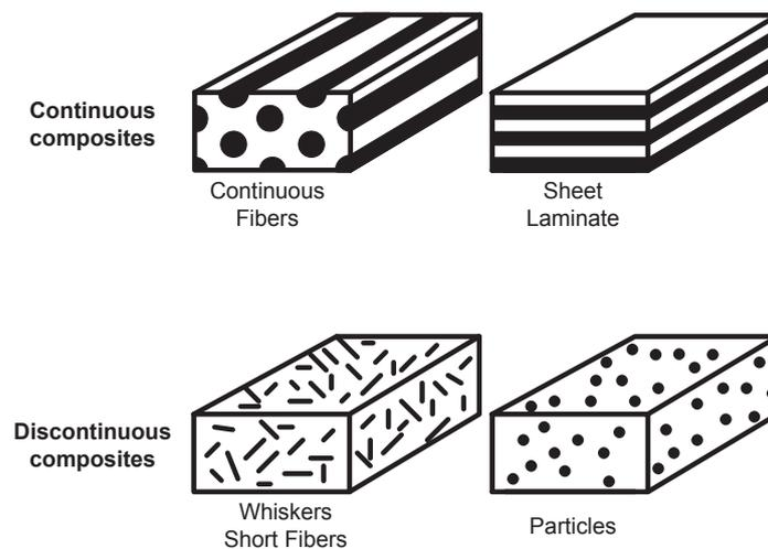
Figure 7: Types of metal matrix composites [CHA2006]
