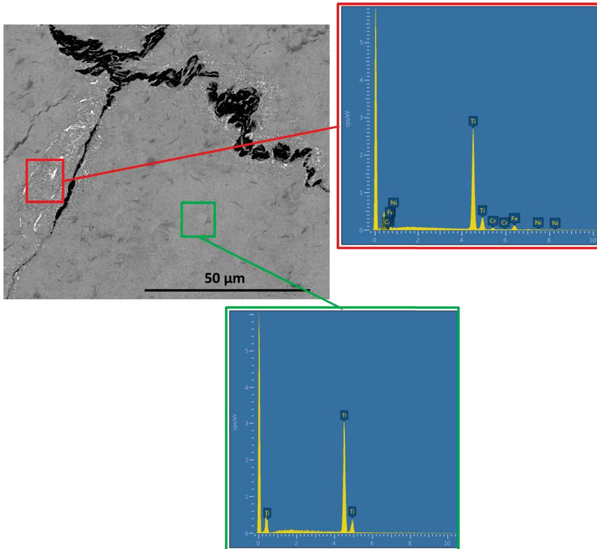
Figure 83: EDX analysis of Ti ball milled, ECAPed for 2 passes with the corresponding BSE micrographs
