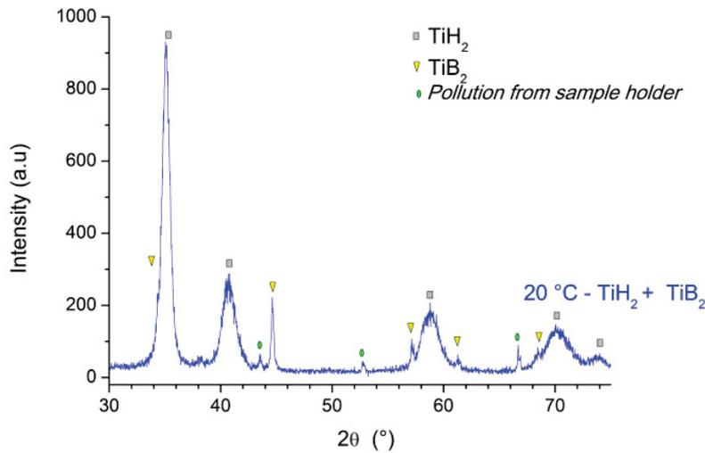
Figure 58: XRD spectrum of TiH<sub>2</sub> - 10vol% TiB<sub>2</sub> after ball mixing
