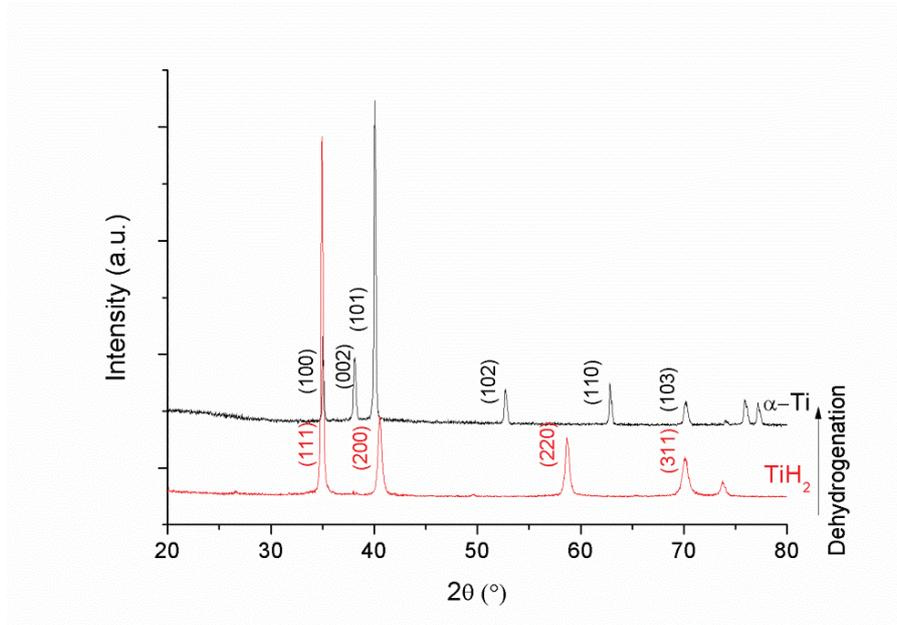
Figure 52: XRD spectra of hydrogenated and dehydrogenated powder
