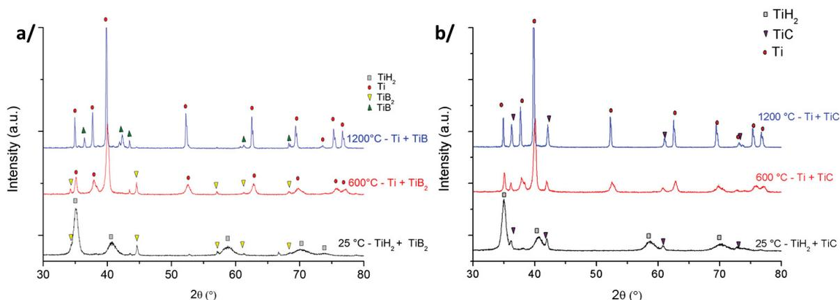
Figure 91: XRD spectra of the pressureless sintering behaviour of a)  $\text{TiH}_2$  - 10%  $\text{TiB}_2$  and b)  $\text{TiH}_2$  - 10% TiC
