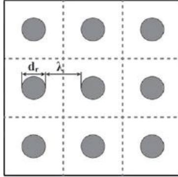
Figure 35: Cubic model for reinforcement distribution [TAN1998]
