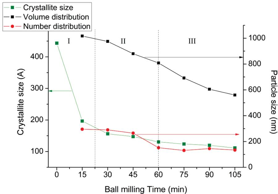
Figure 50:  $\text{TiH}_2$  crystallite size and particle size as a function of ball milling time (green: crystallite in Å, red: particle size number distribution and black: particle size volume distribution in nm)
