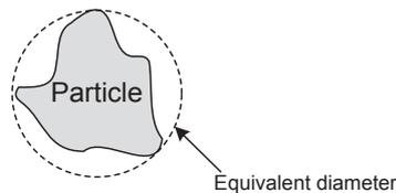
Figure 47: Equivalent diameter of a particle
