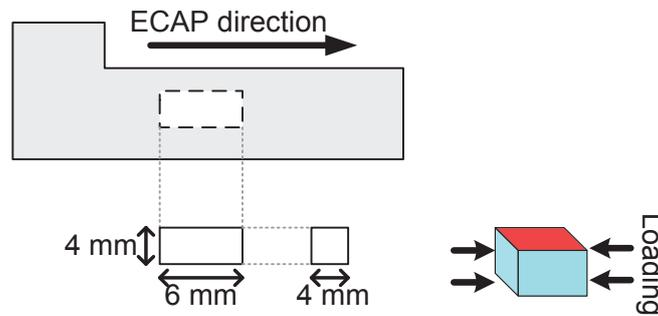
Figure 71: Compression specimen extracted from ECAP sample, with ECAP direction
