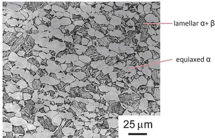
Figure 6: Bimodal microstructure of Ti-6Al-4V (SEM) [NAL2002]
