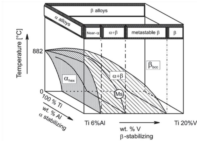
Figure 4: 3D phase diagram of Ti alloys classification [LEY2003]
