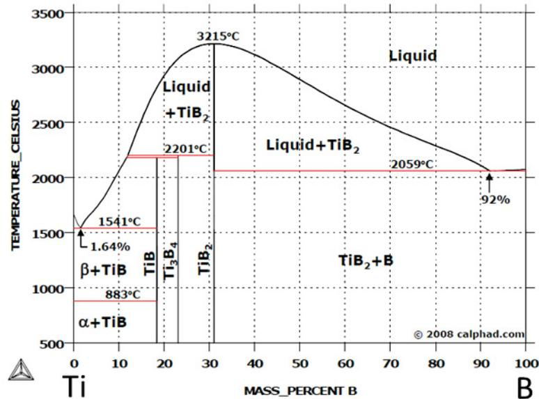
Figure 11: Titanium-Boron Phase Diagram [CAL2008]
