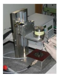
Fig. 2.1: Piezoelectric axial vibrator; device for atmospheric pressure rheology
