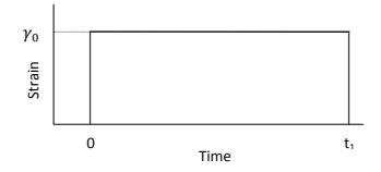
Fig. 1.12: Application of constant strain to study stress relaxation response in Maxwell model
