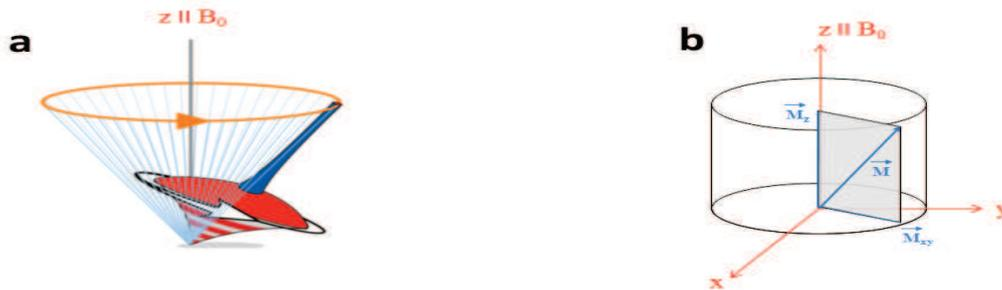
**Figure 1.1.** Following application of a radio frequency (RF) field  $B_1$ , the net magnetization  $M$  is tipped away from the longitudinal direction (a). The resulting vector has both longitudinal  $M_z$  and transverse  $M_{xy}$  components (b)
