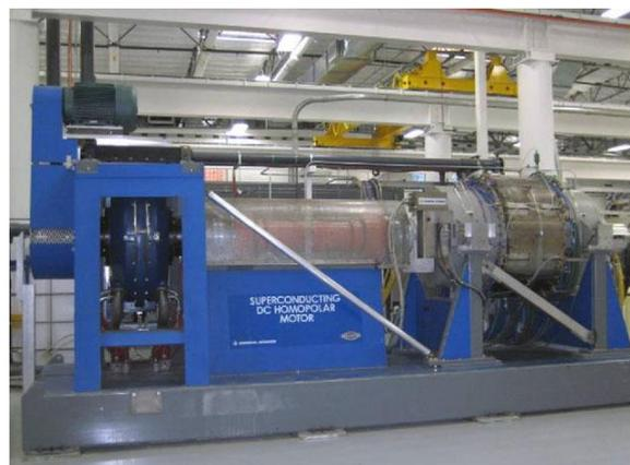
Figure I-26: Moteur Homopolaire 3,7 MW, GENERAL ATOMICS [Ref]
