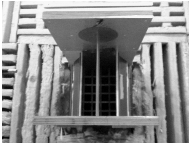
Figure 4.6.: Experimental setup showing the airfoil mock-up mounted vertically and the wind tunnel nozzle in the anechoic chamber of ECL.
