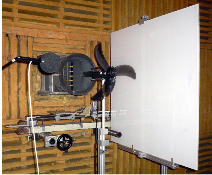
Figure 5.14.: Experimental axial fan-scattering screen configuration in the anechoic chamber.
