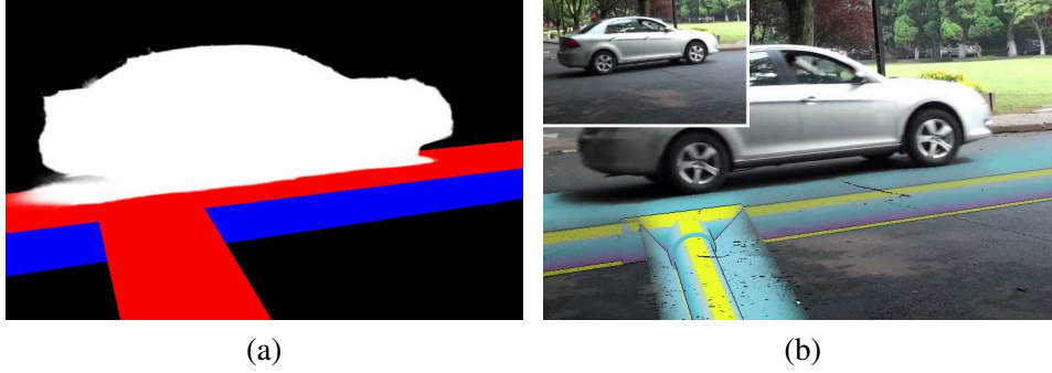
Figure 3.2: Depth-ordered segmentation (a) for the result using tunnel-based cutaways (b), the original image is on the top left corner. The red and blue regions are respectively the main and second focus region. The blue region corresponds to the cut geometry in front of the virtual object. Context cues are extracted from the video outside the white region that is the moving objects: they are in front of the virtual object.
