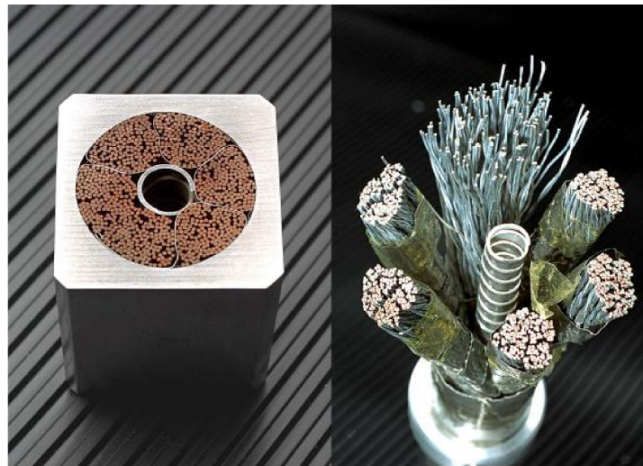
Figure 23: Two ITER CICCs, on the left, the CS model coil CICC, on the right the ITER TF model coil conductor
