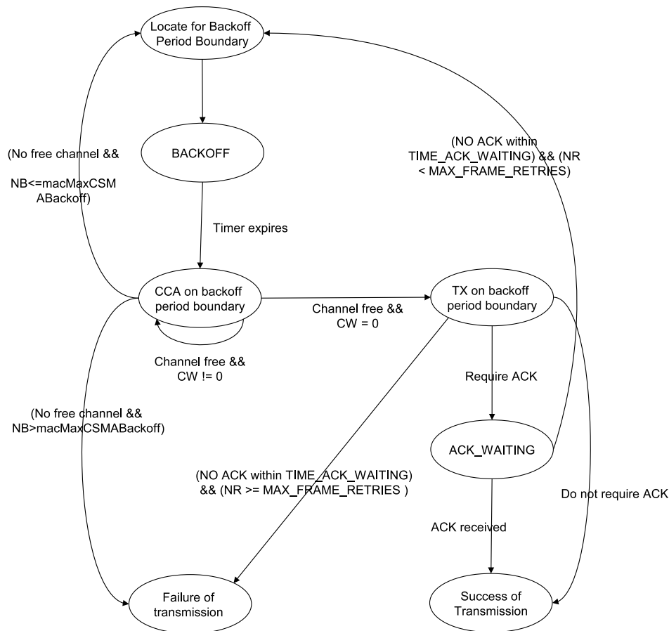
FIG. 3.8: State machine for microcontroller of IEEE 802.15.4 MAC protocol
