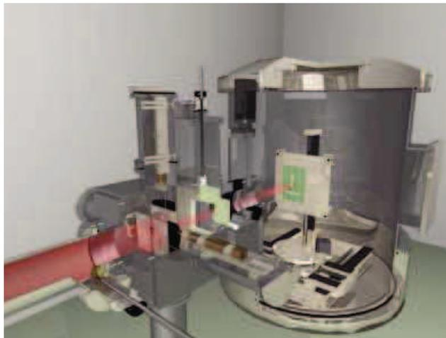
**Figure 1.24:** Heavy ion irradiation chamber installed at university of Jyväskylä, Finland. The linear movement apparatus allows position and tilting adjustments.
