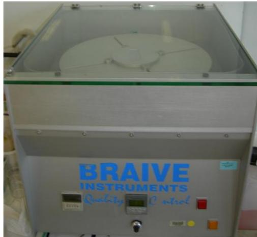
**Figure 2- 1** : Spin-coater Braive Instrument.
