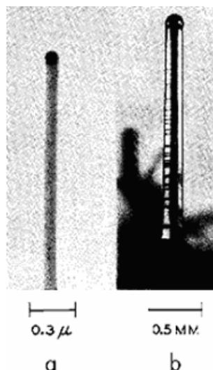
Fig.2.1.1 Silicon filament from Wagner and Ellis<sup>3</sup>
