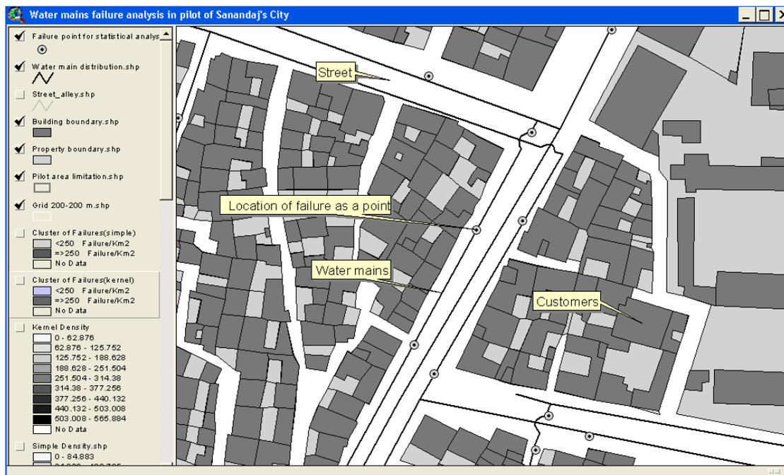
Fig. 2.21 Observed failure locations on water pipelines network and related GIS layers
