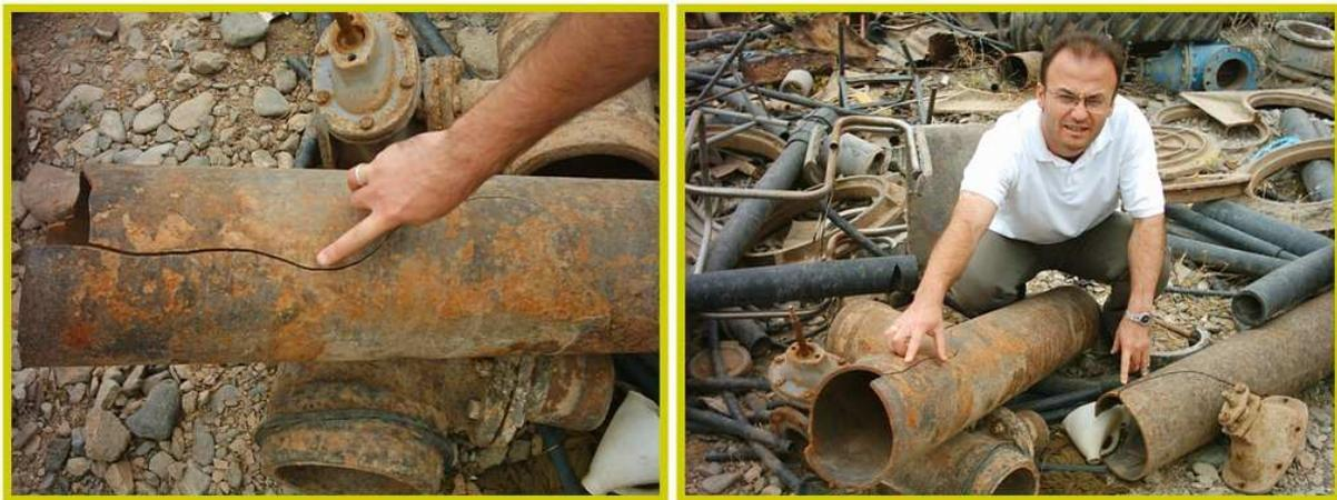
**Fig. 1.4 Spiral breaks on cast iron in study area (closely inspection)**
