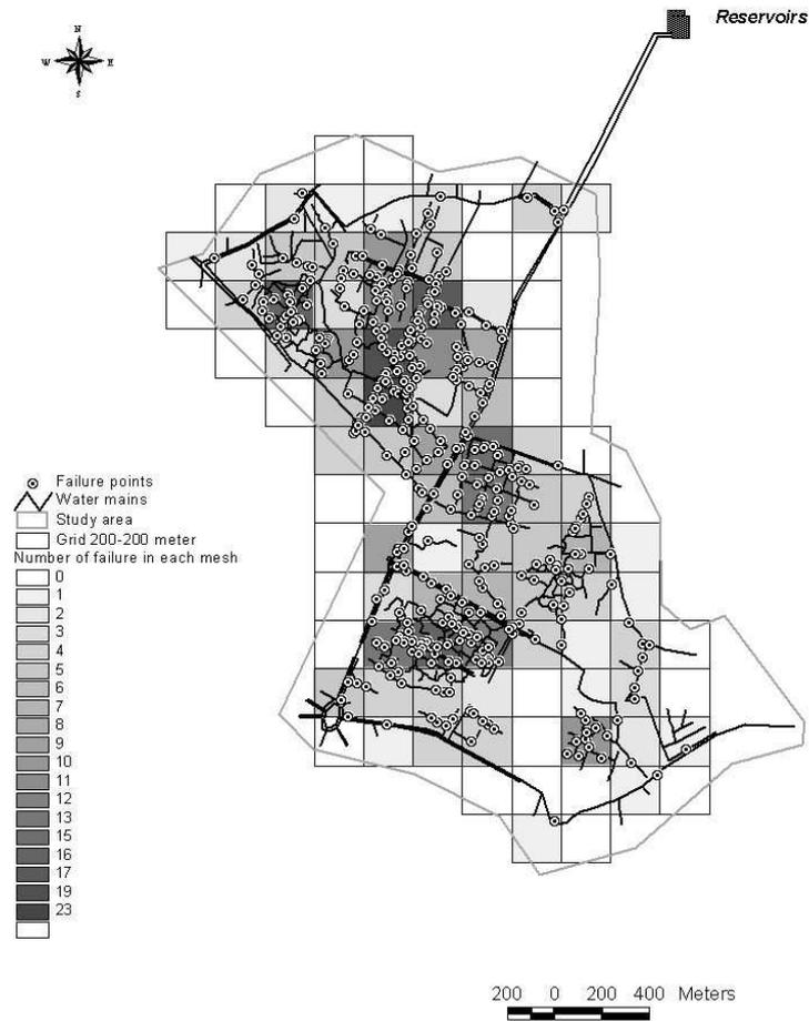
**Fig. 2.29** Number of water pipelines failure point in each cell
