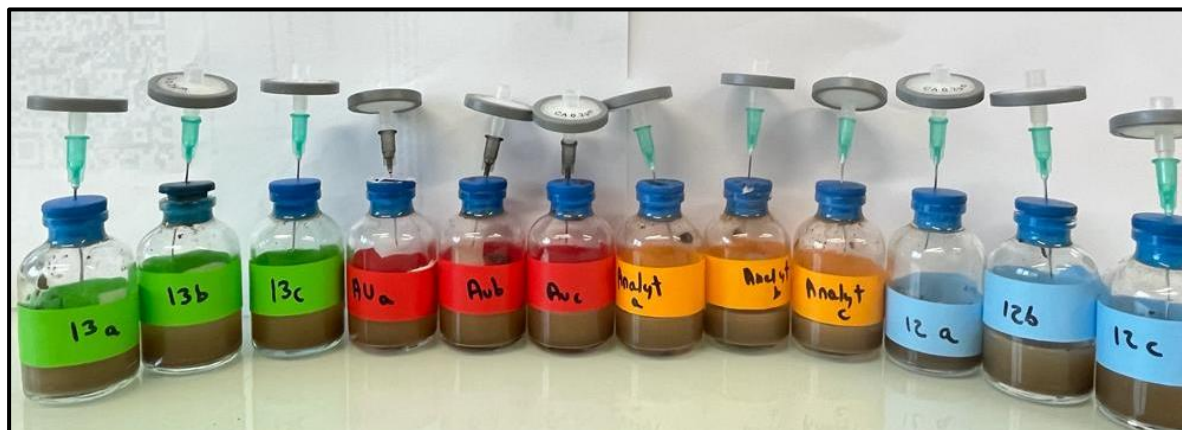
Figure 3.5. Oxic microcosms for stable isotope probing experiments.
