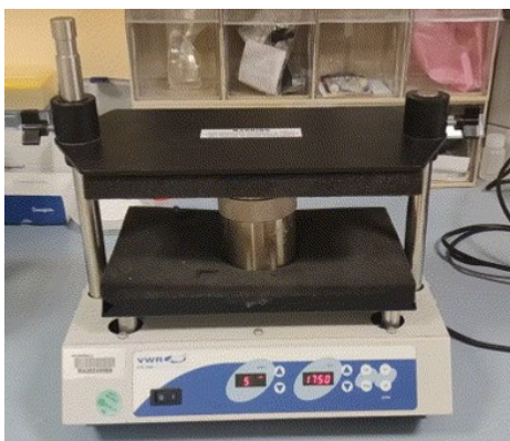
Figure II.27: Photograph of the setup employed for generating mixing inside the hydrothermal vessel. On this picture, the hydrothermal vessel is fixed between two plates which shakes the vessel horizontally.
