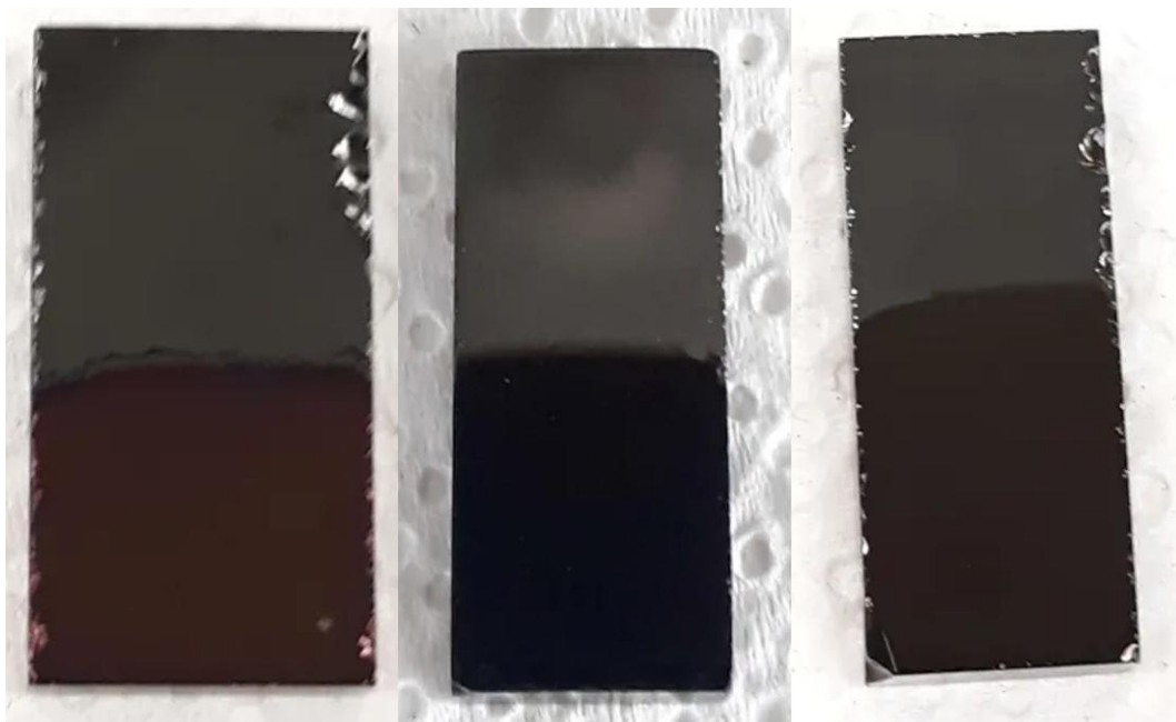
Figure 51. Pictures of the deposited films on carbon plate working electrodes after 25 CV cycles at 20 mV/s (a), 200 mV/s (b) and 1000 mV/s (c)
