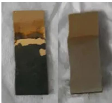
Figure 42. Pictures of films of 1,8-DHN co-deposited with \text{CuCl}_2 with 25 CV cycles at 20 mV/s (left) and 200 mV/s (right).
