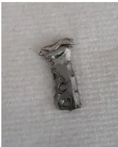
Figure 38. Picture of the Co-Cr piece after 1,8-DHN film deposition (dark part).
