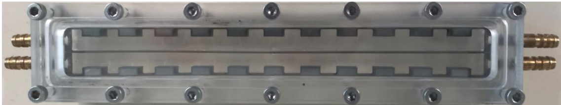
Figure 6.2: Fabricated (a): TO-optimized, (b): Benchmark and (c): Simplified HX units using the water jet cutting process.
