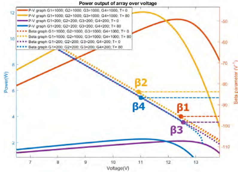
Figure 3.8: Graph displaying the value of \beta parameter when operating at MPP for four conditions of temperature and irradiance. Irradiance of the four PV modules (G1, G2, G3, G4) are given in Wm^2 and their temperature T is given in ^{\circ}C .
