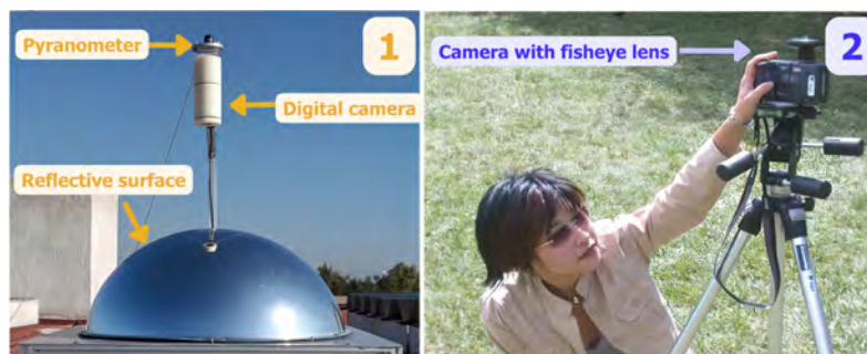
Figure 1.8: Reflective dome technique (1) [31] and fisheye camera imaging (2) [32]
