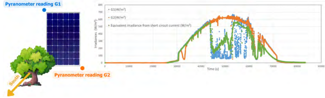
Figure 1.25: Result snippet to highlight the difference between the effective received by a solar panel and pyranometer reading due to the presence of shadows.
