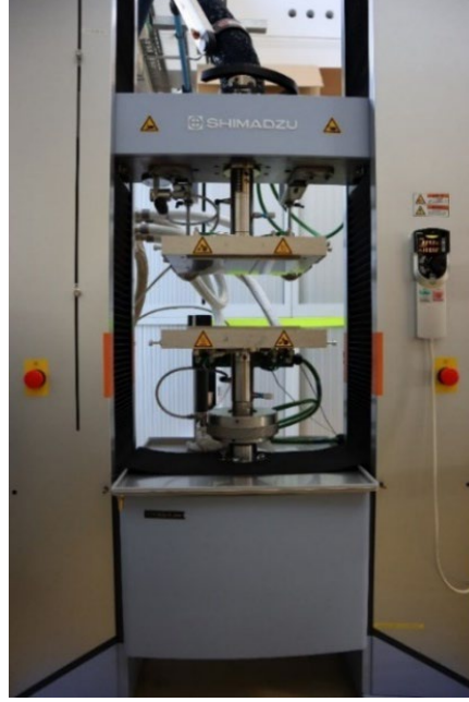
Figure 4.9: Compression testing machine Shimadzu Ag-Xplus.
