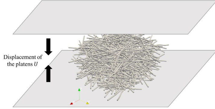
Figure 3.9: Through-thickness compaction of a stack of fiber bundles between two moving platens.
