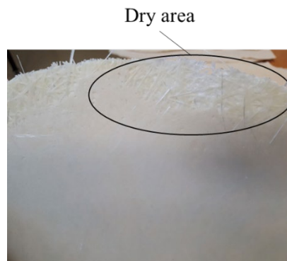
Figure 2.36: Dry area at the flow front.
