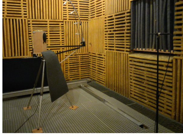
Figure A.3 – Setup used for directivity measurement, with loudspeaker on the left and microphone on the right. (Microphones mounted on a circular stand at the top of the image are not used.)
