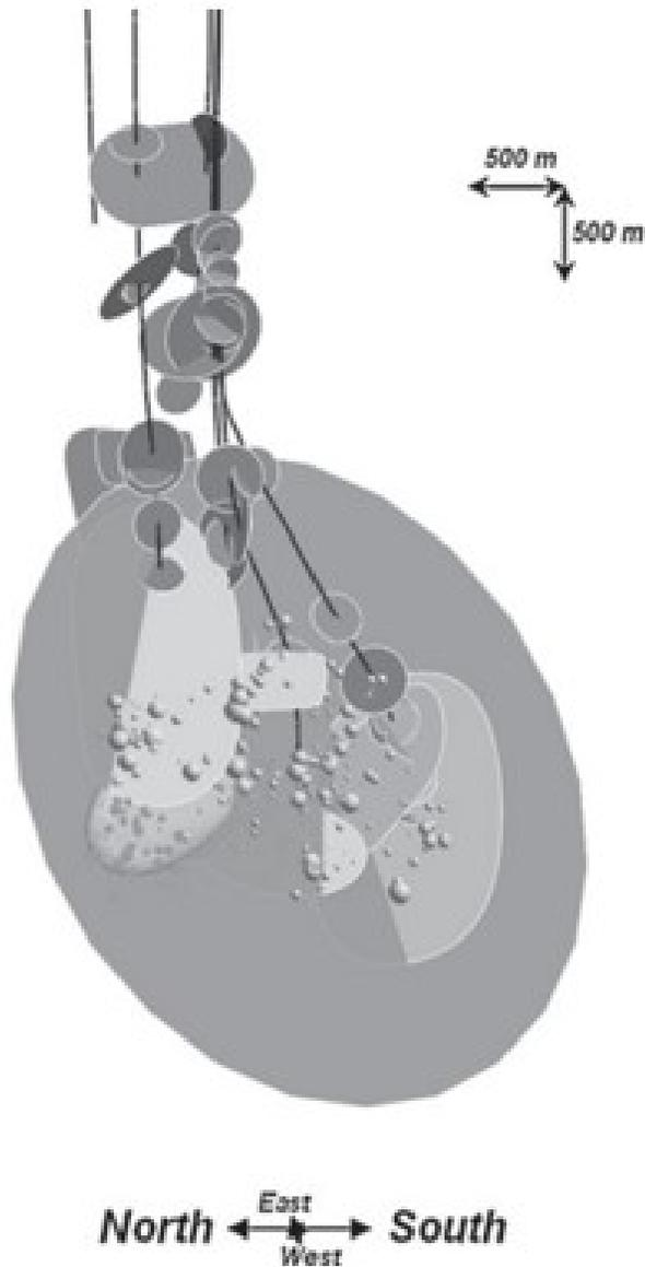
Figure 1.4: 3D view of the induced seismicity in Soutz-Sous-Forêts, modified from (Sausse et al., 2010); The circles indicate seismic events
