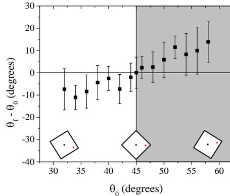
FIG. 4. Rotation of no-legs intruders released at different attack angles close to 45 degrees, specifically from 32 to 58 (or -32). Points represent average values over 10 repetitions and error bars show their standard deviations.
