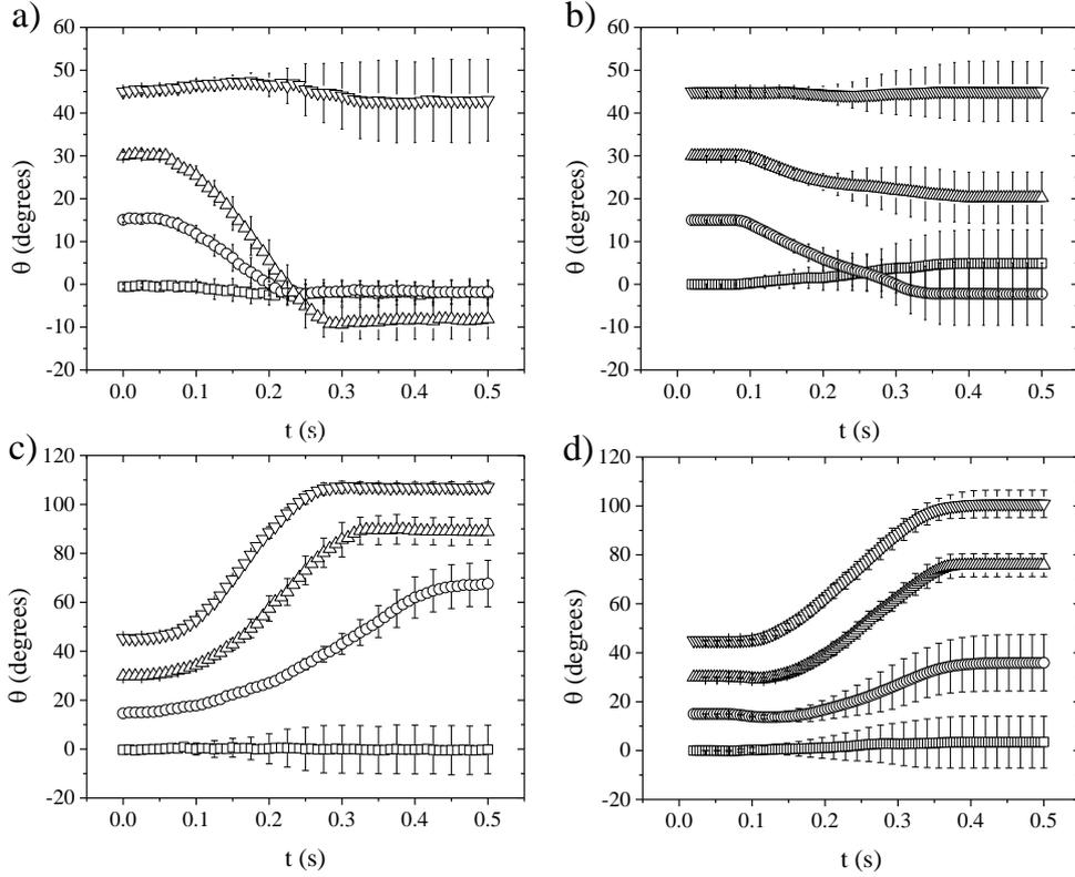
FIG. 3. Rotation with different initial orientation angles. Time evolutions, (a) experimental and (b) numerical for no-legs intruders and (c) experimental and (d) numerical for two-legs intruders.  $\theta$  is measured from the horizontal. Each curve shown is averaged over 10 repetitions and bars represent its standard deviations.
