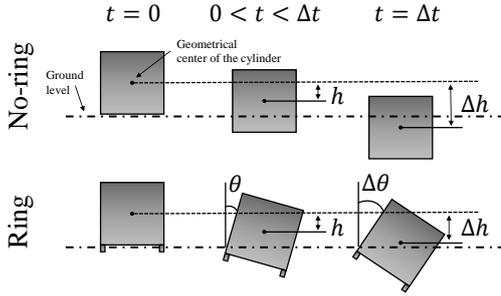
FIG. 2. Sketch of sinking and tilting processes. The top row illustrates the sinking process of a No-ring cylinder in three moments during the experimental interval from  $t = 0$  to a final time  $t = \Delta t$ . The bottom row shows the same temporal sequence for a Ring cylinder, which tilts in addition to sink.
