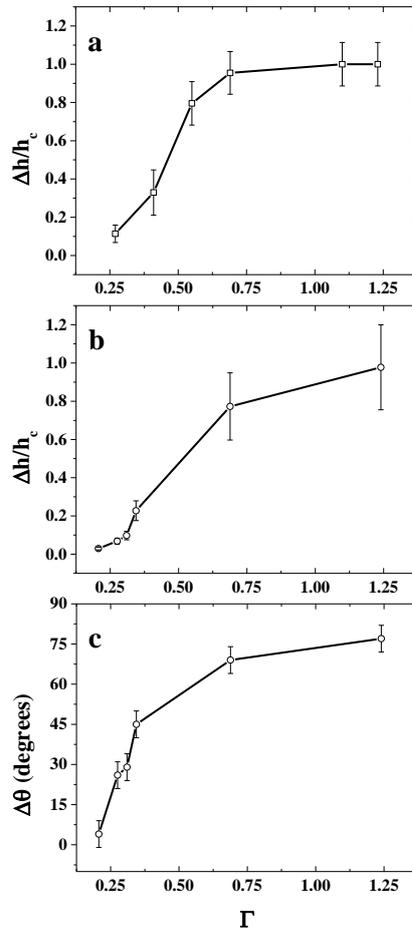
FIG. 7. Experiments. Sinking and tilting: heights and angles for different dimensionless accelerations  $\Gamma$ . Final sink heights for No-ring cylinders (a) and for Ring cylinders (b). Final tilt angles for Ring cylinders (c). Tilt angles of No-ring cylinders are not shown for the same reasons of the previous figure.
