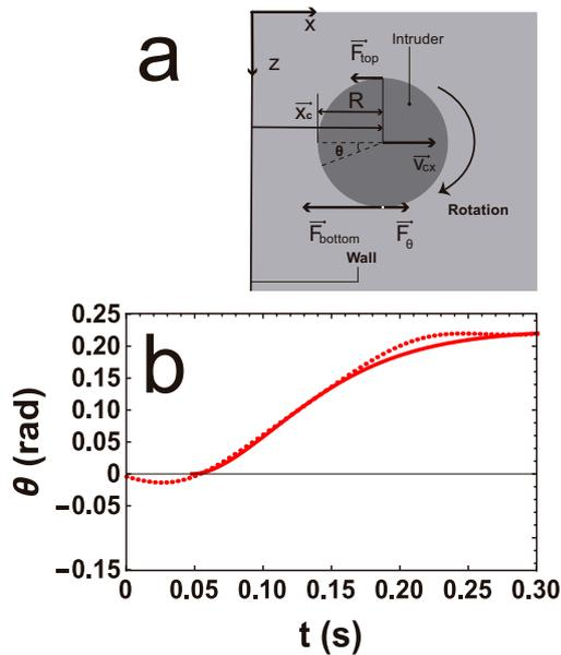
FIG. 2. Preliminary modeling of rotation. (a) Sketch representing the main parameters and forces involved in modeling the intruder's rotation. (b) Rotation vs time for  $x_0 = 0$  cm: circles and line represents experiment and the output of the equation  $\dot{\theta} = k_r \dot{x} \exp(-z/\lambda) - f_\theta \theta$  (see main text for details).
