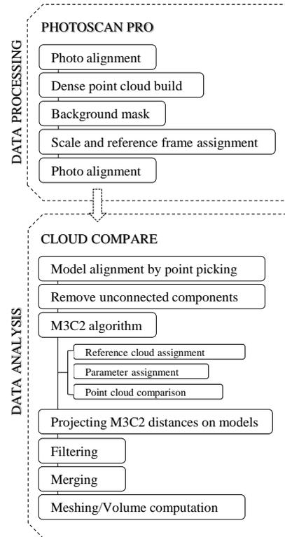
FIG. 3. Generalized workflow for data processing (dune reconstruction) and analysis (change detection).
