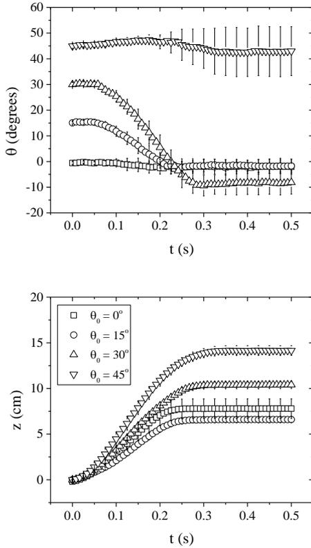
FIG. 2. Time evolution of the (a) the orientation angle and (b) of the vertical displacement  $z$  of intruders released at different attack angles. Each curve shown is averaged over 10 repetitions and bars represent standard deviation from the mean.
