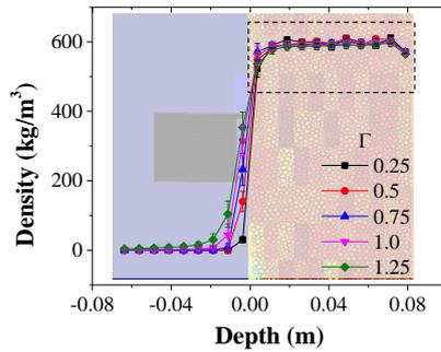
FIG. 17. (color online) Density profiles for the different values of dimensionless acceleration  $\Gamma$  obtained from the simulations. The background shows the subdivision of the simulation box where the color of each rectangle goes sequentially from blue to red and represents its density. The intruder is represented in light gray.
