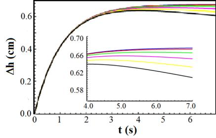
FIG. 16. (color online) Time dependence of sinking depth as calculated solving numerically Eq. (A.12) considering the variation of  $S$  and  $D$  provoked by tilting (see text). Upper curve is for  $\theta_{max} = 0$  while the lower one is for  $\theta_{max} = \pi/3$ . Between them,  $\theta_{max}$  varies in steps of  $\pi/15$ . The inset shows the last three seconds.
