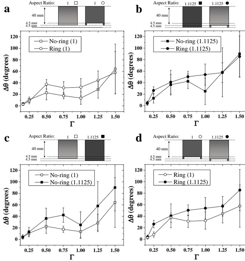
FIG. 14. Simulations. Final tilt angles at different  $\Gamma$  for two intruders with (a) aspect ratio 1 and different foundations; (b) aspect ratio 1.1125 and different foundations; (c) a flat bottom and different aspect ratios and (d) a ring at the bottom and different aspect ratios.
