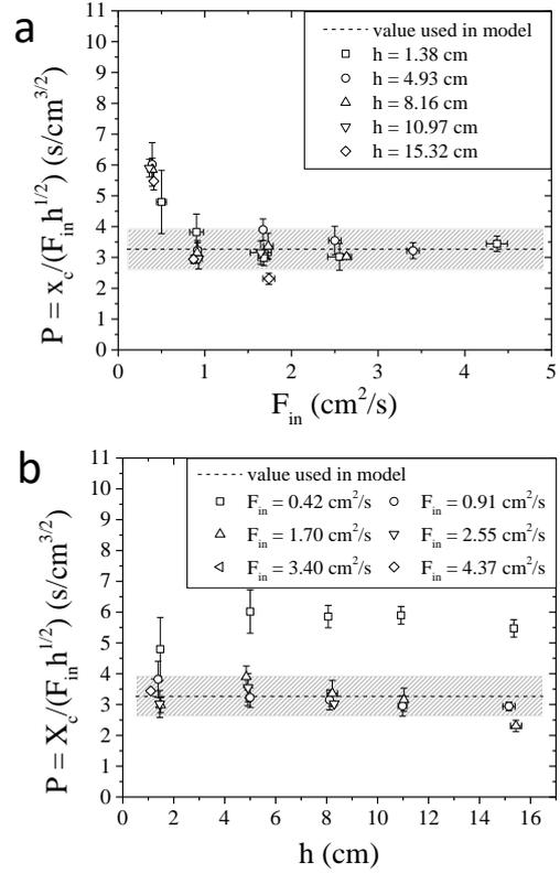
FIG. 4. Quantitative comparison between experiments and model. Dependence with the input flux (a) and with the deposition height (b) of the proportionality constant in Eq. (3),  $P$ . Black dashed lines represent the value of  $P = X_c/(F_{in}\sqrt{h})$  used in our model to reproduce the experimental data and the height of the gray rectangles represents its standard error.  $P_{model} = 3.27 \pm 0.65 \text{ s/cm}^{3/2}$ .
