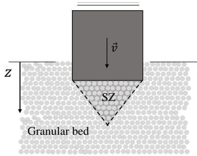
Figure 1: Stagnant zone (SZ). The system includes the intruder and a conical SZ ahead of it
